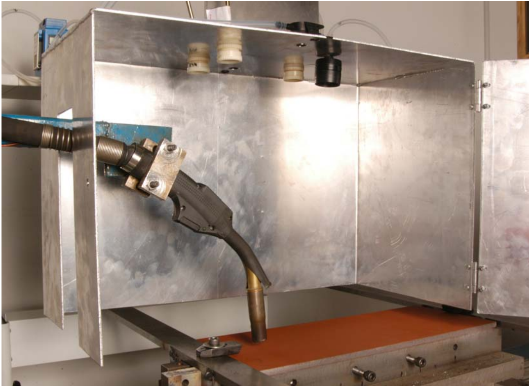
Figure 1: Welding Test Hood with Sampling Devices in Position
