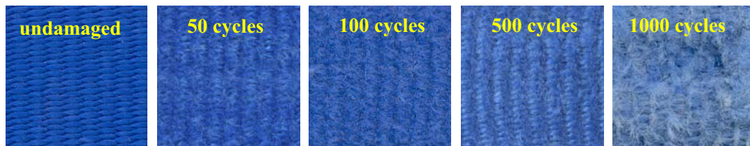
Figure 5. Showing the progression of damage from abrasion over concrete
