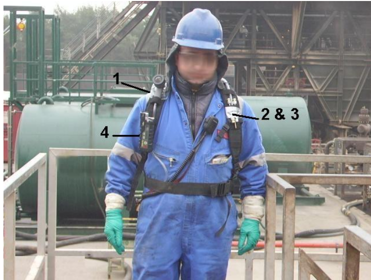
Figure 1. Arrangement of Samplers During Personal Sampling
