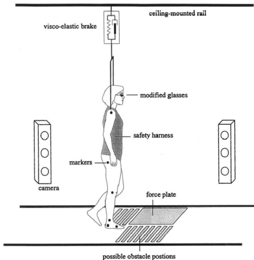
Figure 3 Schematic diagram showing a generic trip study experimental set-up, including a walk way, force plate, trip hazard, fall arrest system, motion capture markers, and video cameras [after Pijnappels et al.].
