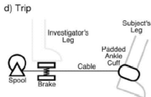
Figure 4 Schematic diagram of the cuff method of inducing trips as used by Smeeters et al [after Smeeters et al.].
