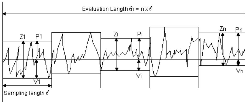
The Rz surface roughness parameter is defined as the mean of the sum of Zi within each sampling length over the entire evaluation length.
