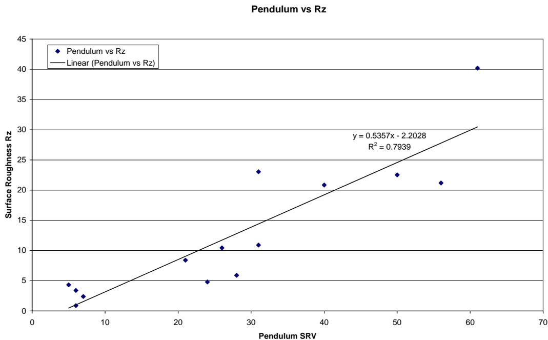
Figure 3.1 Graph showing wet pendulum values plotted against Rz surface roughness.
