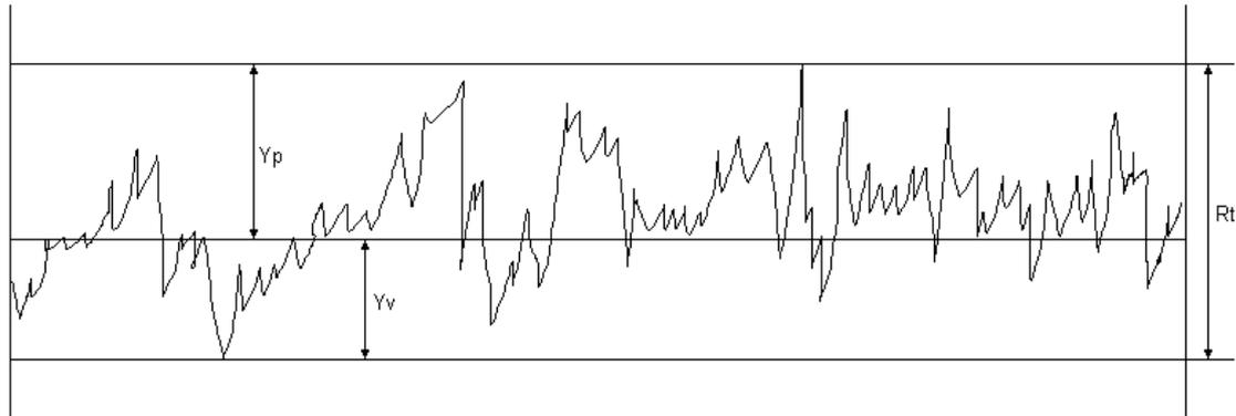
Diagram showing a schematic representation of how  $R_t$  is calculated.
