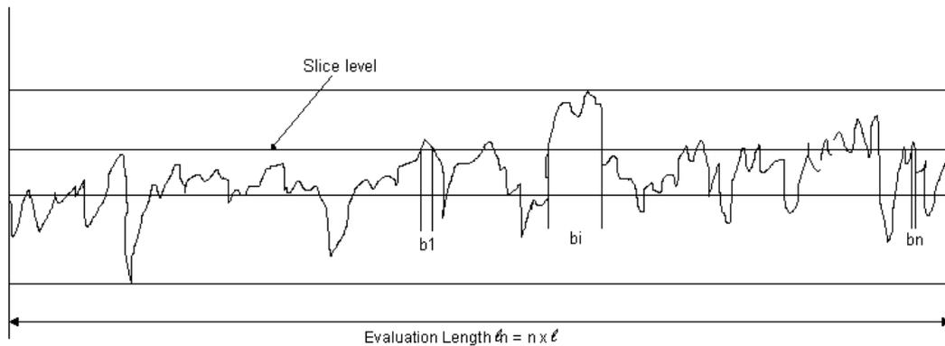
Schematic diagram showing how  $R_{mr}$  is calculated
