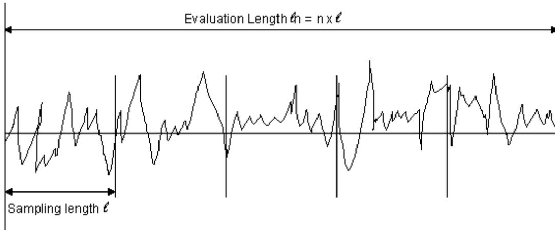
Diagram showing schematic representation of surface roughness trace.
