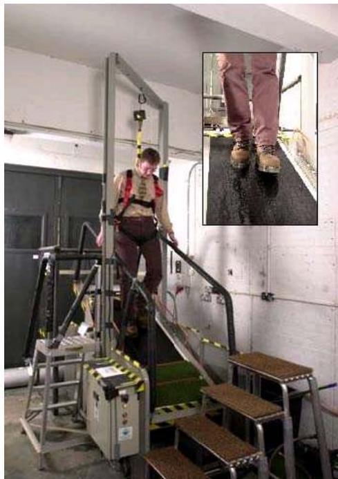
Figure 2.3 The ‘HSL-PS-SOP-12’ ramp-type CoF test.
