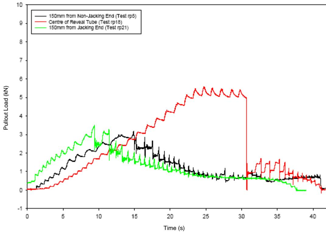
**Figure 41** – Comparison of Effects of Pull tube Location on 2 Turn Reveal Pin Ties Installed in a Concrete Reveal
