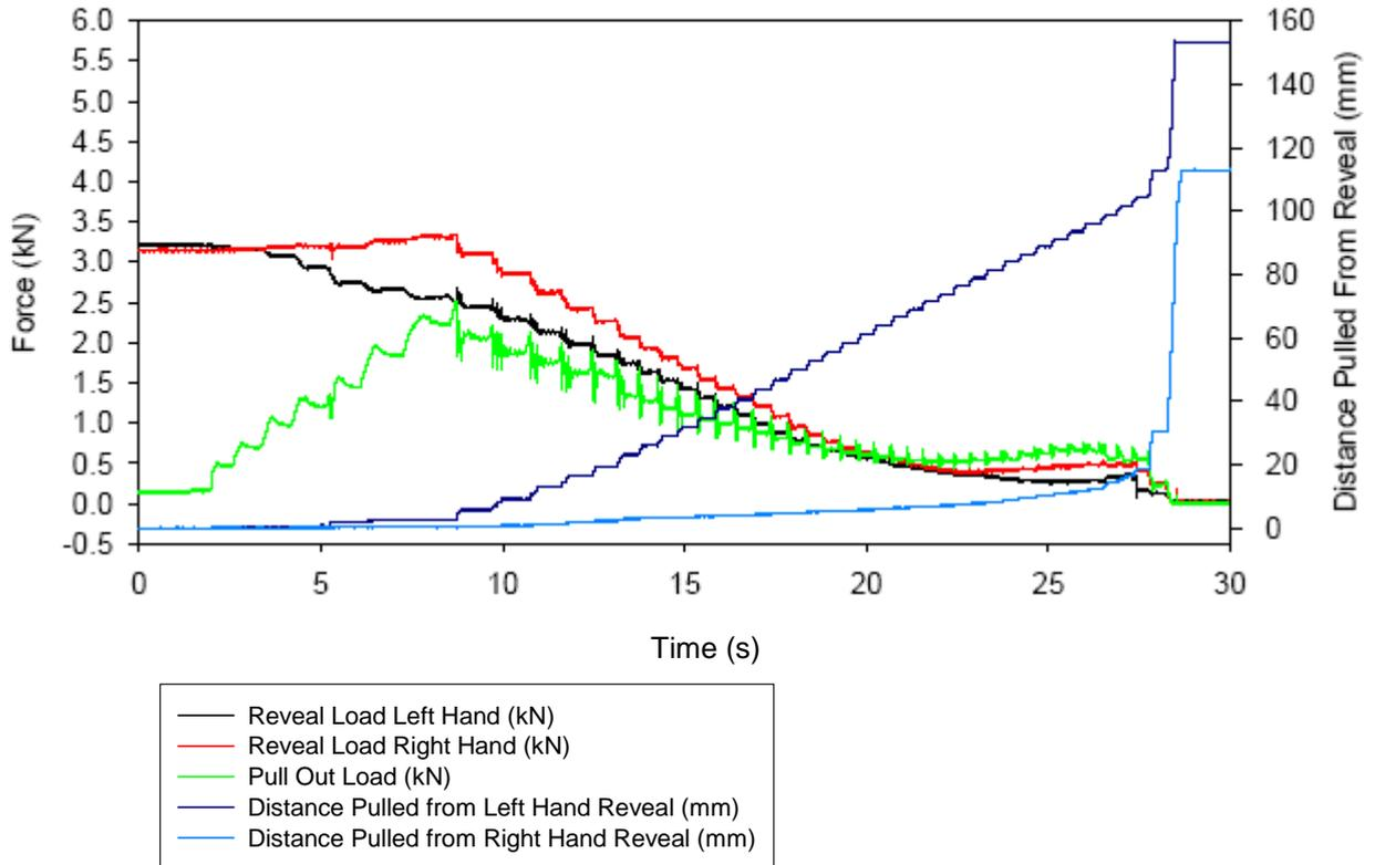
Figures 21 & 22 – 2 Turn Reveal Pin Ties, Pulled 150mm from Non-Jacking End, Moist Packing, 10 minutes bedding-in
