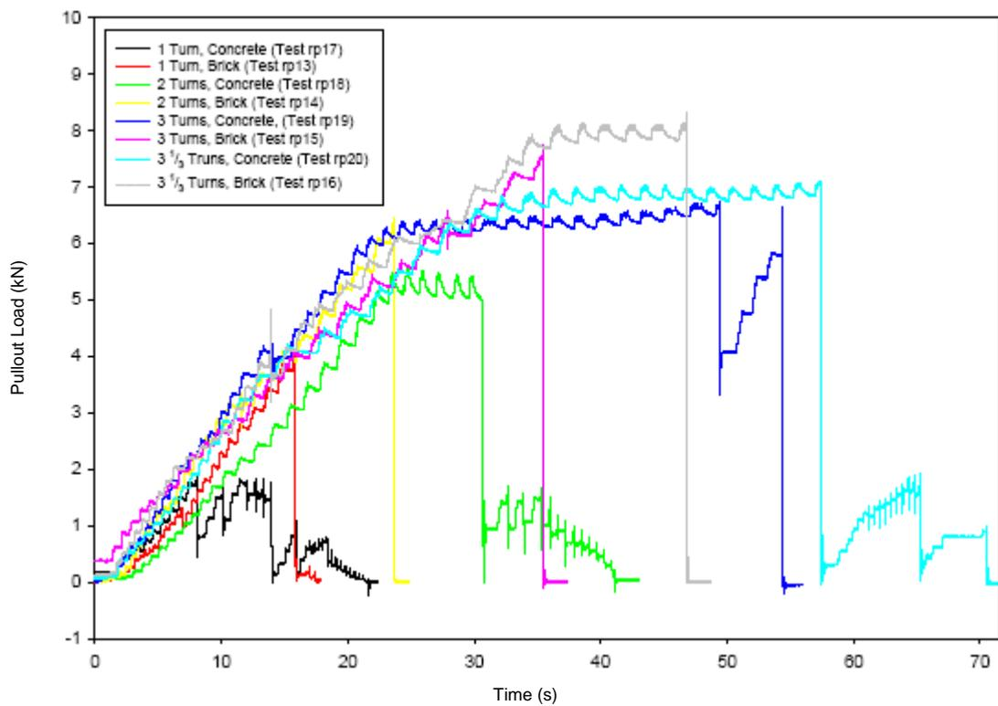
**Figure 40** – Comparison of Centrally Pulled Reveal Pin Tie Tests
