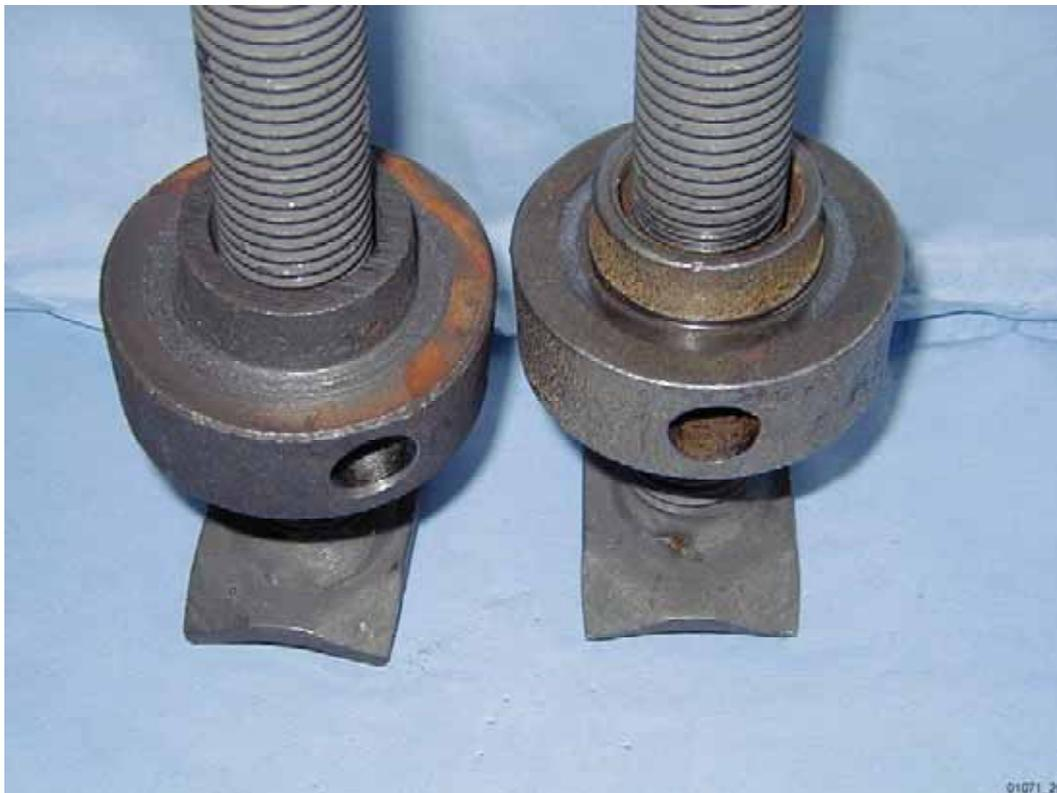
**Figure 6** – Wear to surface of reveal pin boss
