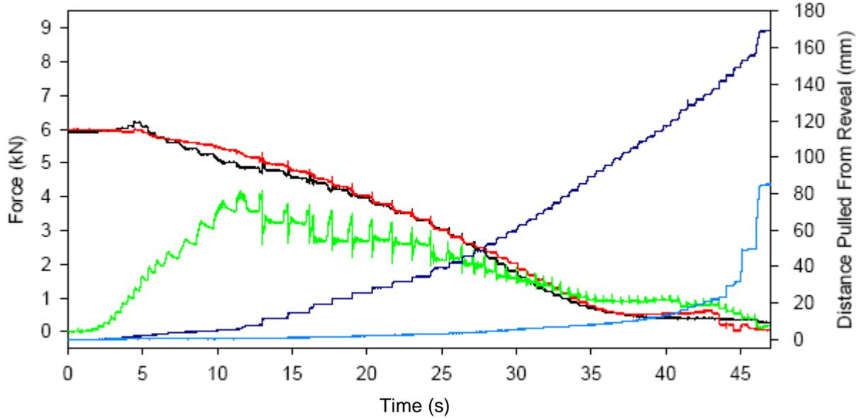
Figure 14 - Test 28, 8.5kN Reveal Load, Reveal Pin Tie, Concrete Reveal,
