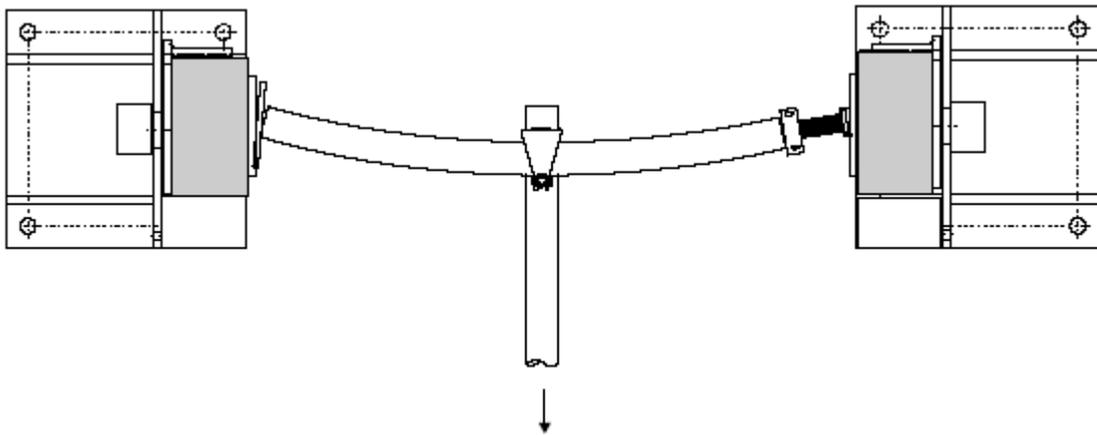
Stage 2 - As the pullout load is applied, the reveal tube bends, increasing the overall length which increases the reveal load
