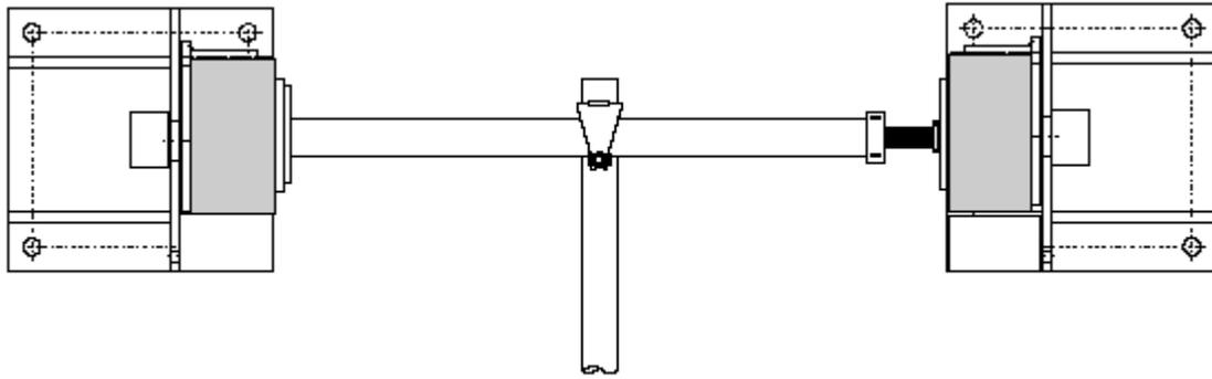
Stage 1 - The tie is tightened into the reveal
