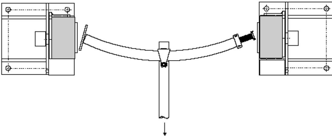
Stage 3 - As the tube continues to bend, it exceeds the critical point where the length starts to decrease and reveal load drops off. As permanent bending occurs, pullout load levels off.
