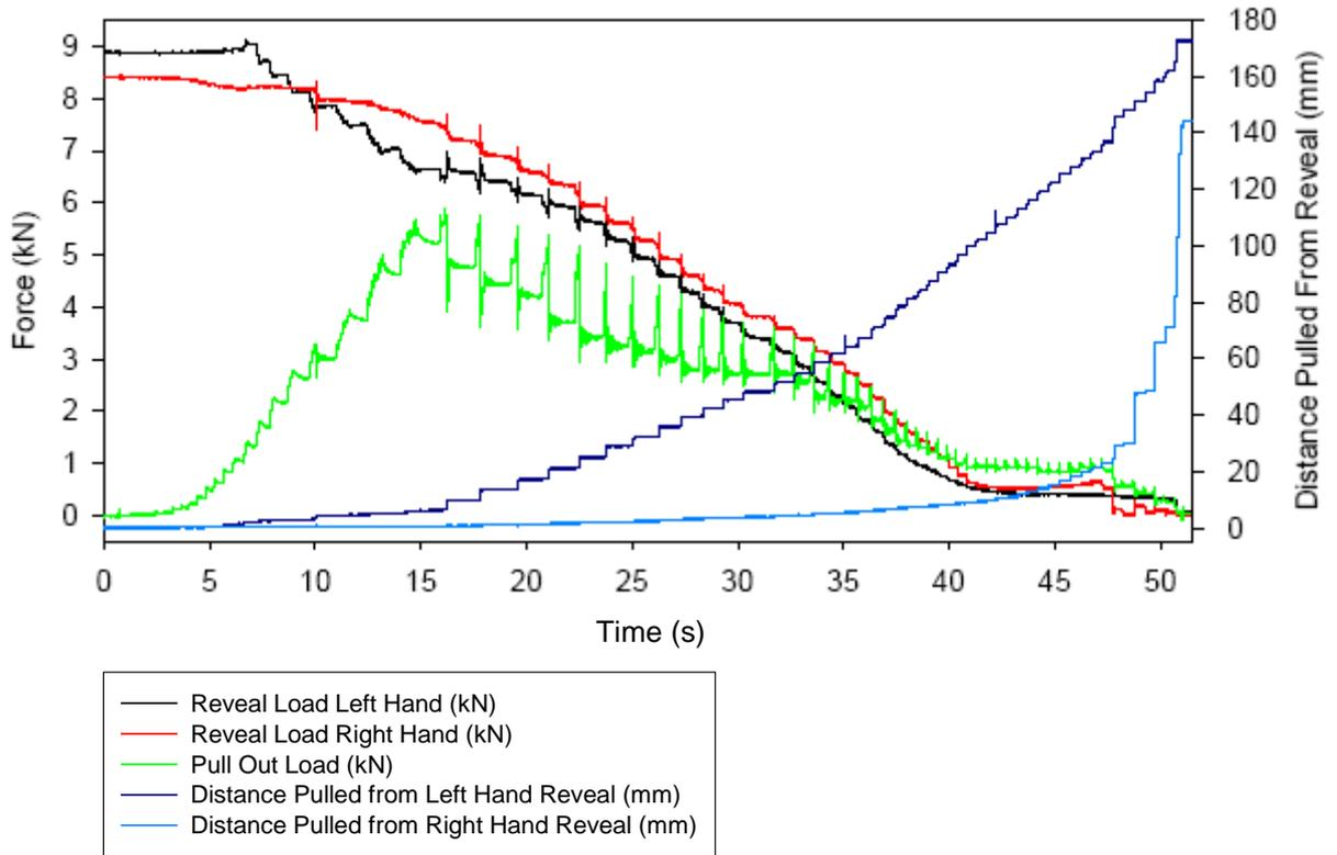
Figures 13 & 14 – 6.0kN & 8.5kN Reveal Load, Reveal Pin Ties, Pulled 150mm from
