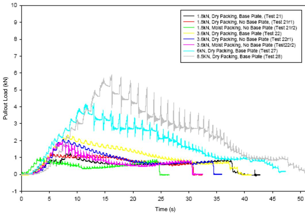
**Figure 37** – Comparison of Reveal Pin Tie installation methods, Pulled 150mm from Non-Jacking End, Concrete Reveal
