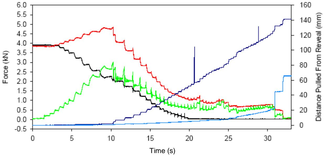
Figure 22 - Test rp10, 2 Turn Reveal Pin Tie, Brick Reveal
