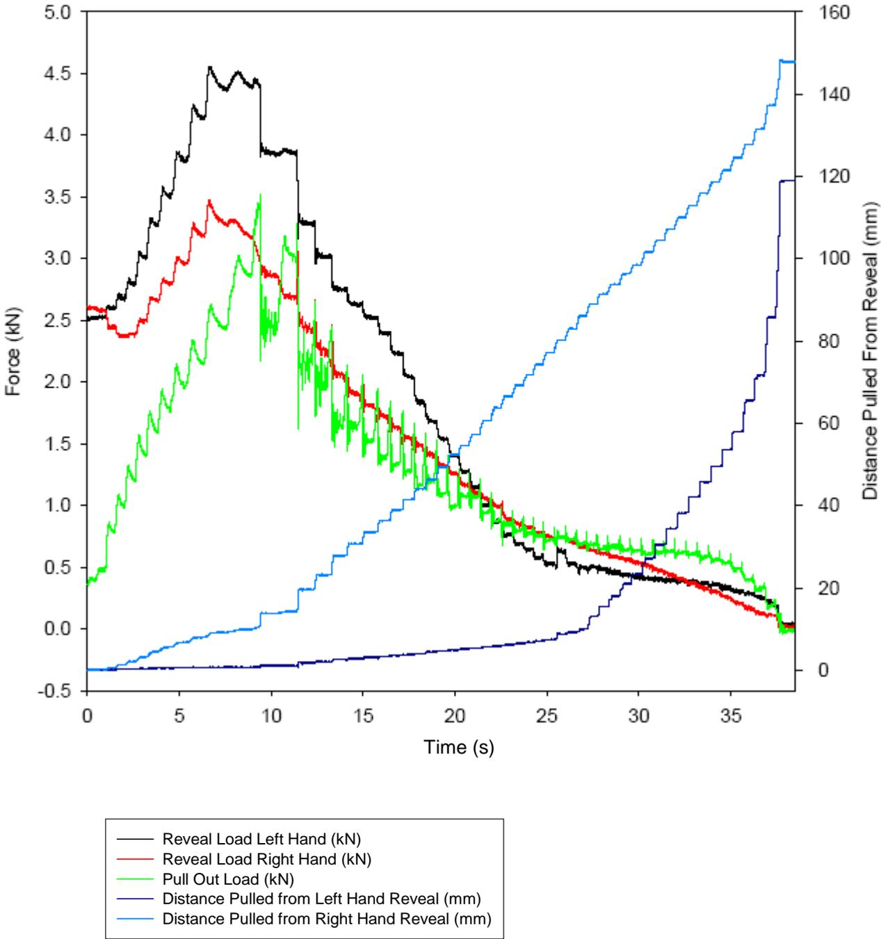
Figure 35 – 2 Turn Reveal Pin Tie, Pulled 150mm from Jacking End, Moist Packing, 10 minutes bedding-in
