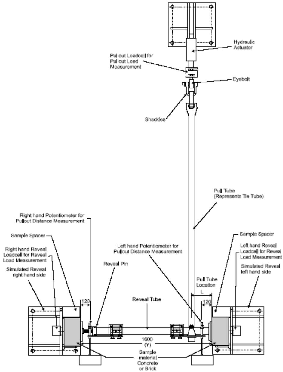
**Figure 2 – Reveal Pin Tie Test Rig Construction**
