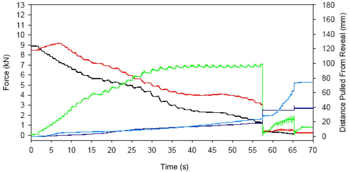
Figure 34 - Test rp16, 3 1/3 Turn Reveal Pin Tie, Brick Reveal
