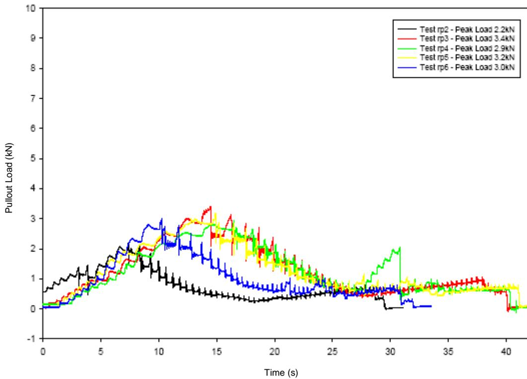
**Figure 39** – Comparison of 2 Turn Reveal Pin Ties Installed in a Concrete Reveal, Pulled 150mm from Non-Jacking End
