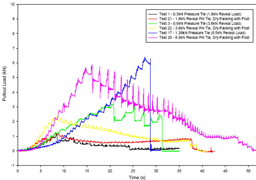
**Figure 42** – Comparison of Pressure Ties with Reveal Pin Ties of Equivalent Reveal Load
