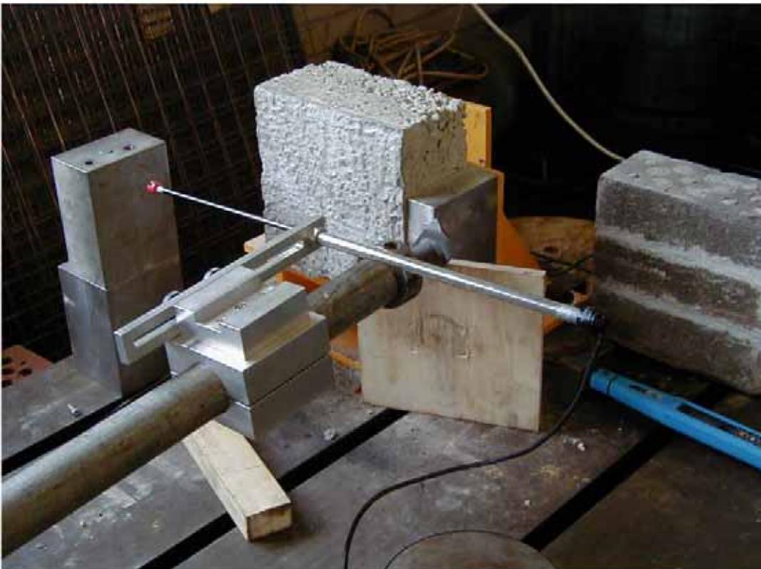
Figure 5(b) - Reveal Pin Tie Failure, Concrete Reveal, Right Hand Side (Test rp18)
