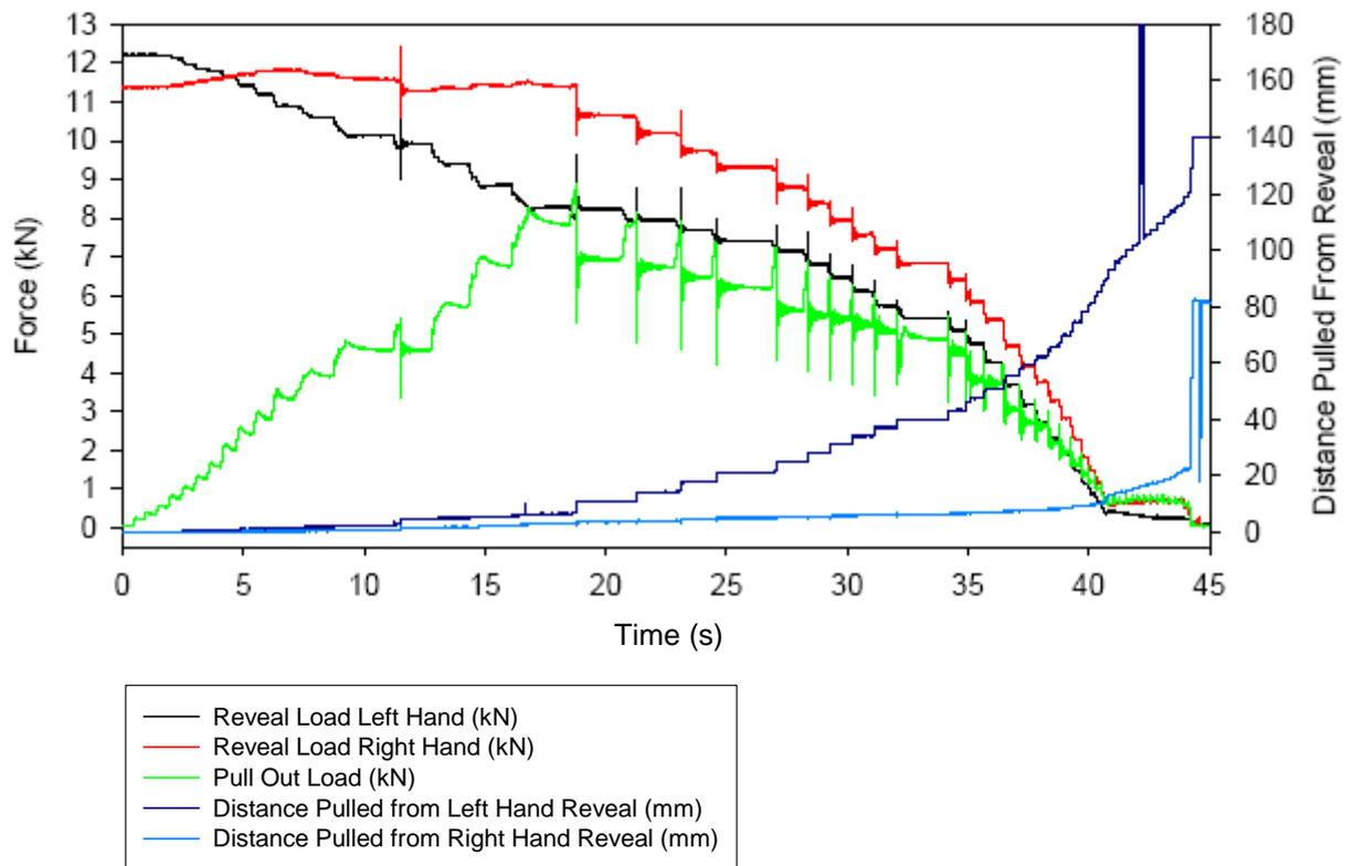
Figures 25 & 26 – 3 1/3 Turn Reveal Pin Ties, Pulled 150mm from Non-Jacking End, Moist Packing, 10 minutes bedding-in
