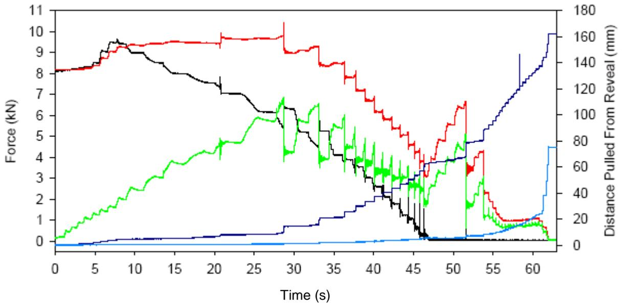
Figure 24 - Test rp11, 3 Turn Reveal Pin Tie, Brick Reveal
