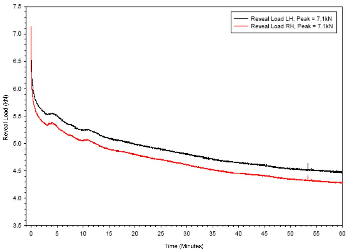
**Figure 44** – Graph Showing Relaxation of 3 Turn Reveal Pin Tie – First Hour
