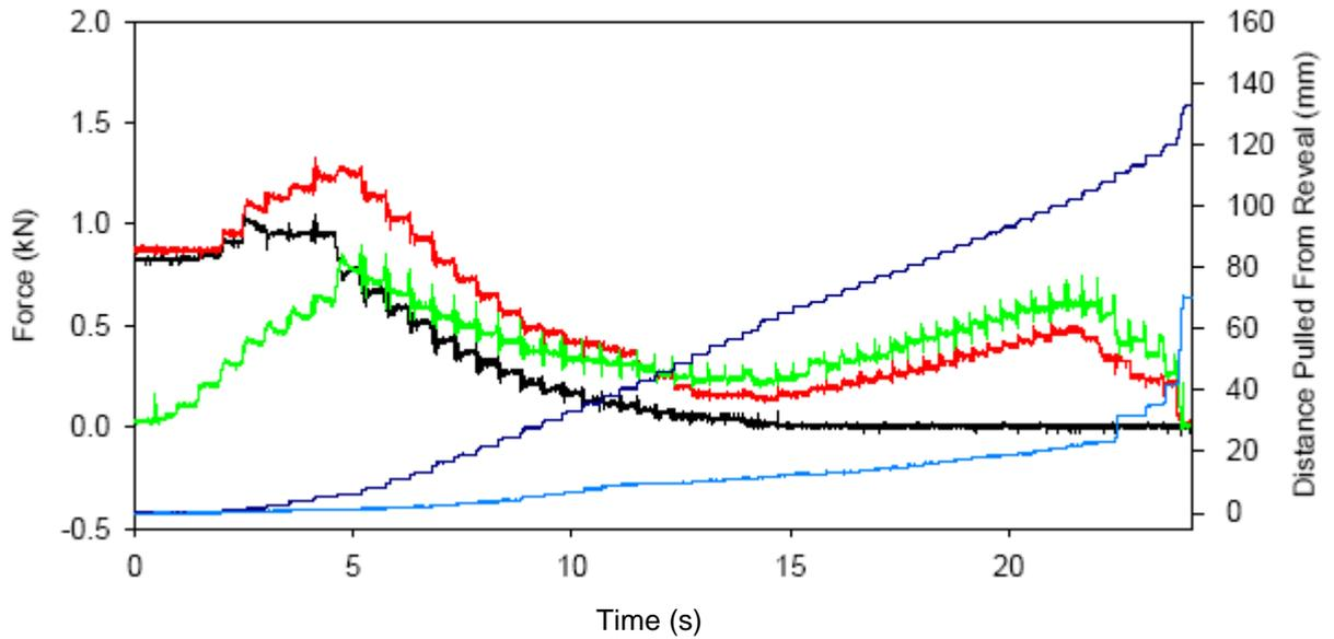
Figure 16 - Test rp9, 1 Turn Reveal Pin Tie, Brick Reveal
