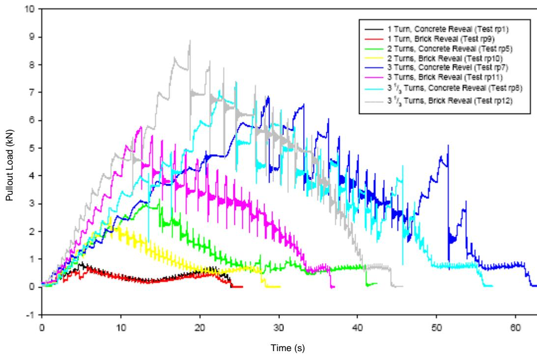
**Figure 38** – Comparison of Reveal Pin Ties Pulled 150mm from Non-Jacking End
