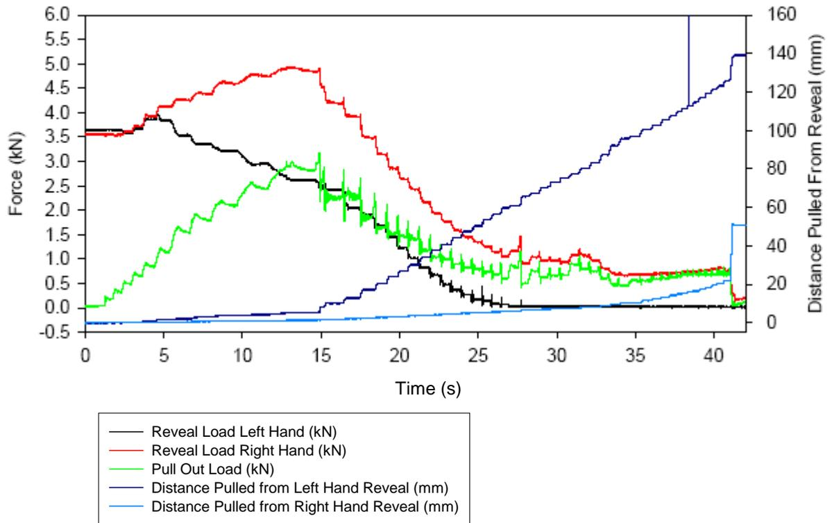
Figures 19 & 20 – 2 Turn Reveal Pin Ties, Pulled 150mm from Non-Jacking End, Moist Packing, 10 minutes bedding-in
