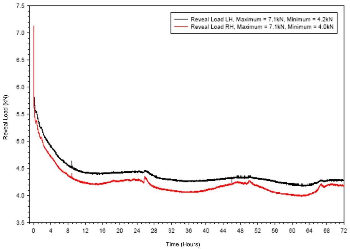
**Figure 43** – Graph Showing Relaxation of 3 Turn Reveal Pin Tie over 3 Day Period
