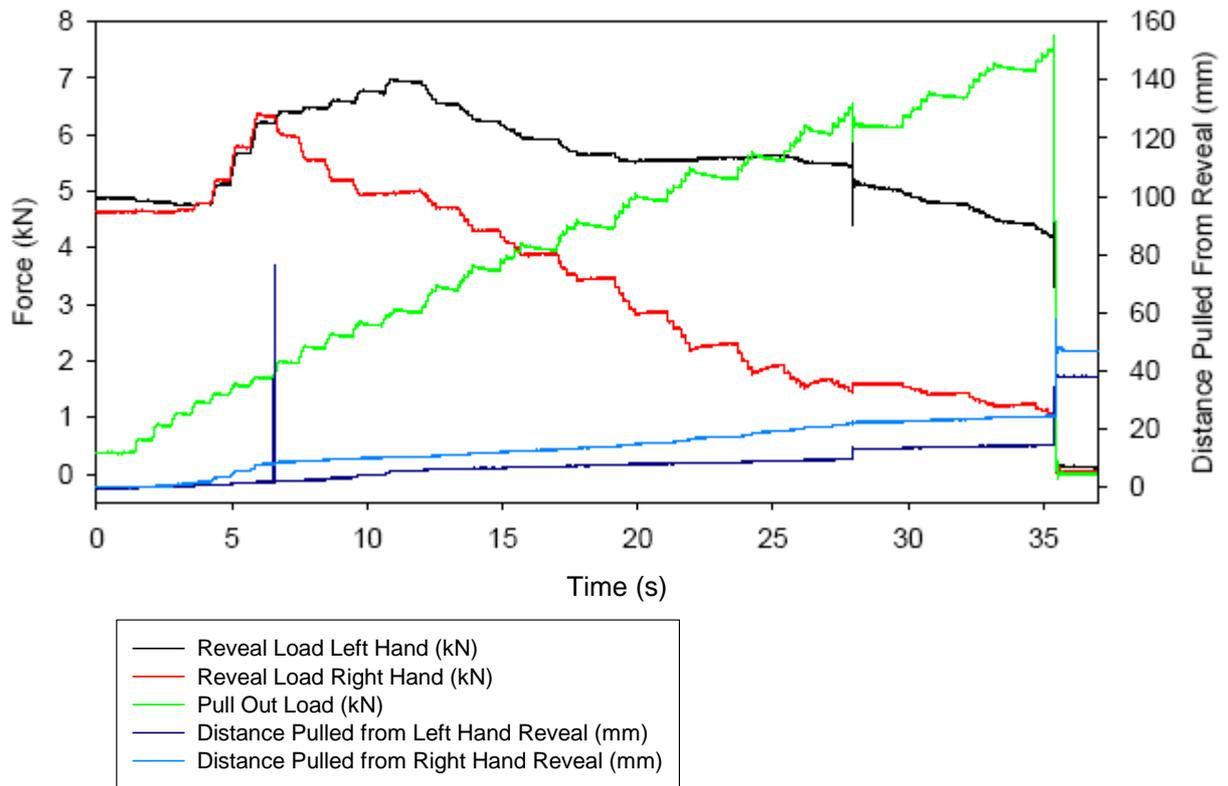
Figures 31 & 32 – 3 Turn Reveal Pin Ties, Pulled from Centre of Reveal Tube, Moist Packing, 10 minutes bedding-in
