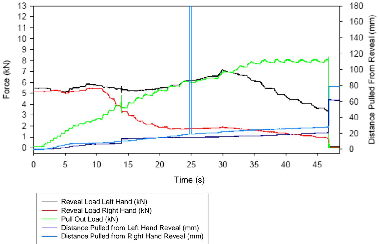
Figures 33 & 34 – 3 1/3 Turn Reveal Pin Ties, Pulled from Centre of Reveal Tube, Moist Packing, 10 minutes bedding-in
