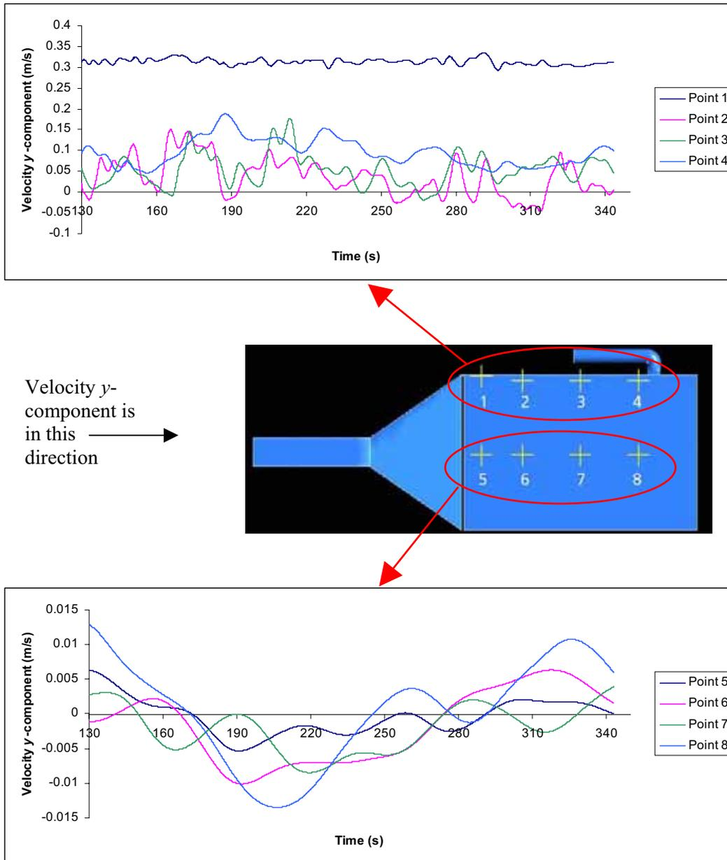
**Figure 5** Variation of the y-component of velocity at 8 monitoring locations for the LES pre-calculation.
