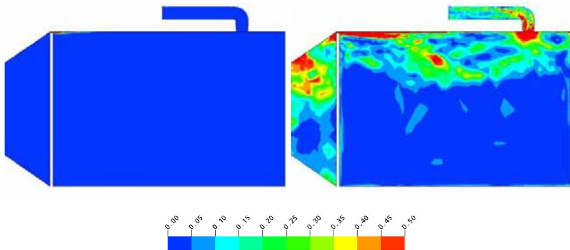
**Figure 12** Contours of the ratio of modelled to total turbulence kinetic energy using the UL calculation method (left) and Pope method (right). Both results are for the LES calculation.
