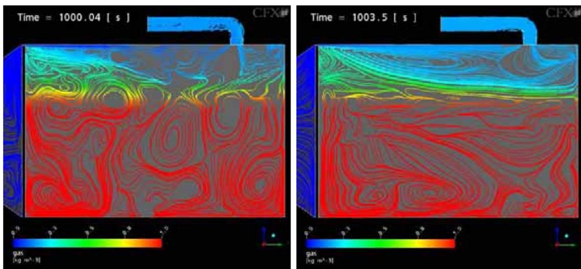
**Figure 7** Streamlines on the mid-plane coloured with the contaminant gas fraction after approximately 1000 seconds from the gas release as predicted by LES (left) and SST RANS model (right). Both results shown are snapshots taken at a single instant in time.
