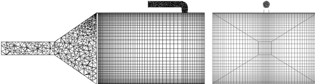
**Figure 3** Side and end views of the computational grid in cross-section.
