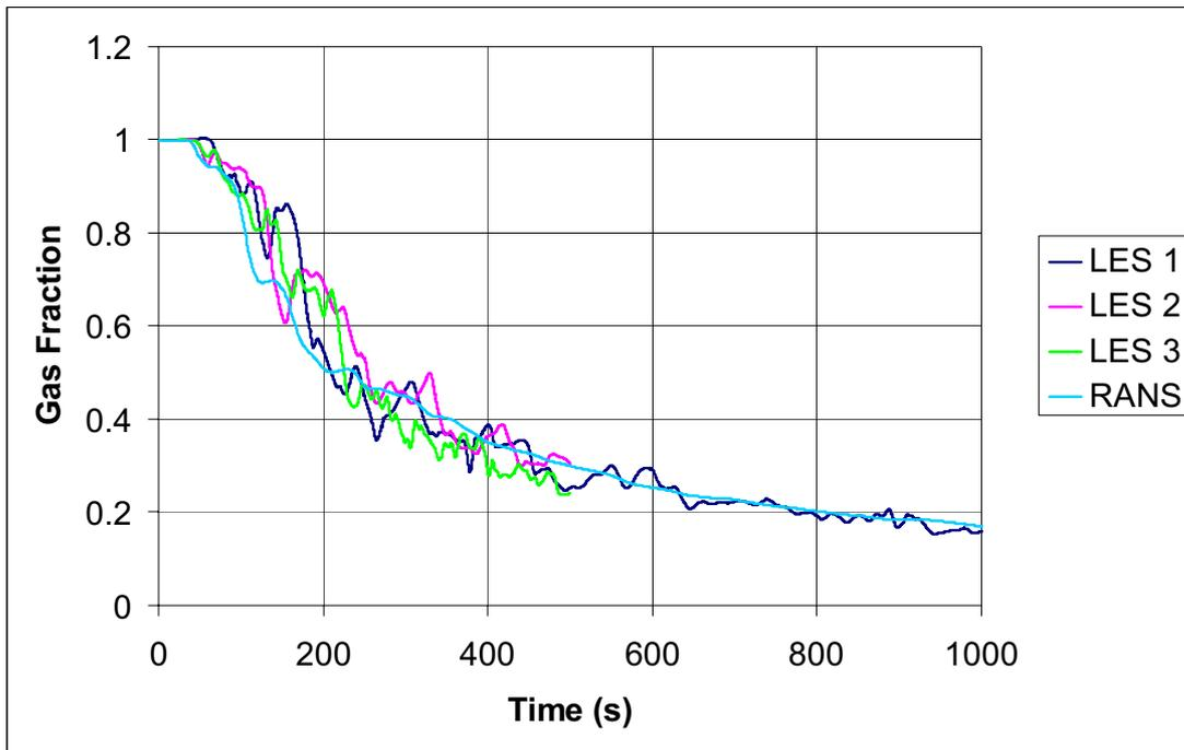
**Figure 8** Variation of the contaminant gas fraction near the exhaust duct over time for three separate LES calculations (LES1, LES2 and LES3) and an SST-model RANS calculation. Calculations LES2 and LES3 were only run for 500 seconds.
