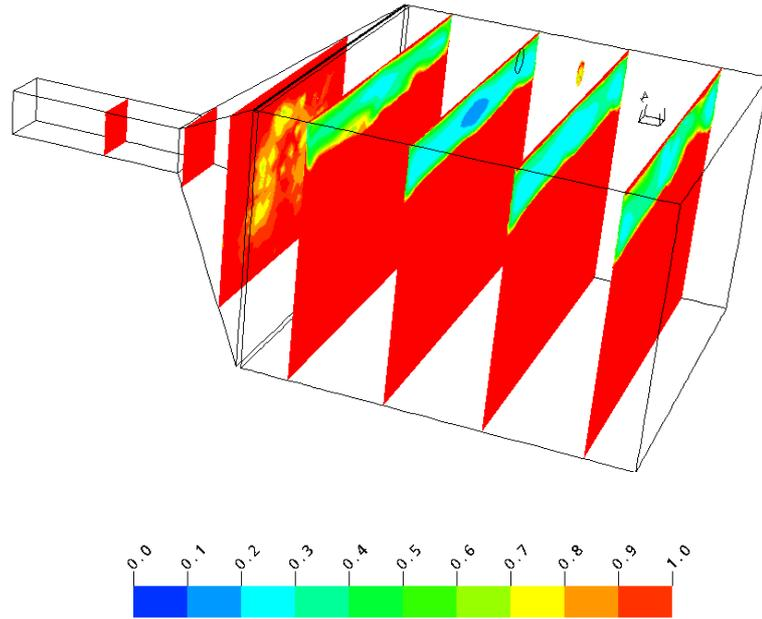
**Figure 9** Contours of the ratio of turbulence length scales to grid cell dimensions for the SST model.
