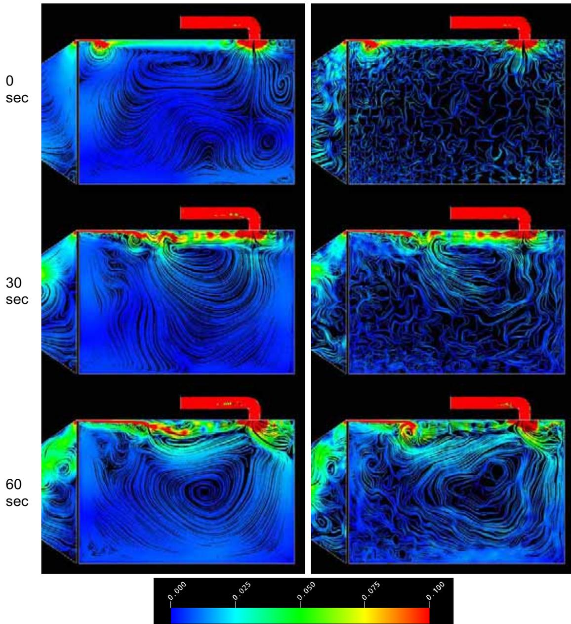
**Figure 4** LES pre-calculations showing the flow development from two different initial conditions; on the left: a pure RANS solution; on the right: the same RANS solution superimposed with 0.01 m/s random fluctuations. Streamlines are shown on the mid-plane of the room coloured with the velocity magnitude.
