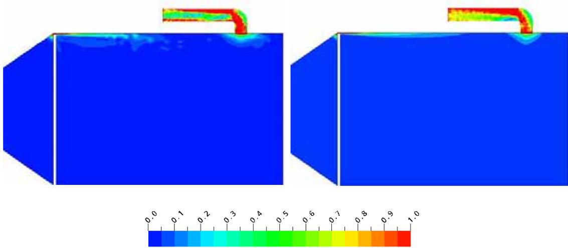
**Figure 11** Contours of the predicted Courant number,  $C$ , on the mid-plane using LES (left) and the SST model (right). In both cases, the time-step used to calculate  $C$  is  $\Delta t = 0.05$  seconds.
