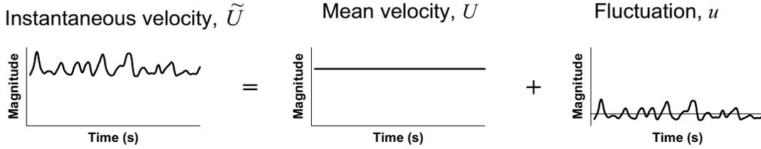
**Figure 1** Decomposition of the instantaneous velocity field,  $\tilde{U}$ , into the mean,  $U$  and fluctuation,  $u$ .
