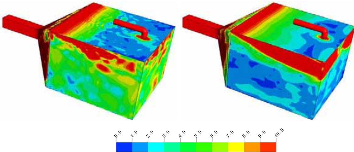
**Figure 10** Dimensionless wall-normal distances ( $y^+$ ) for the LES (left) and the SST model (right). Both results shown are for a single instant in time.
