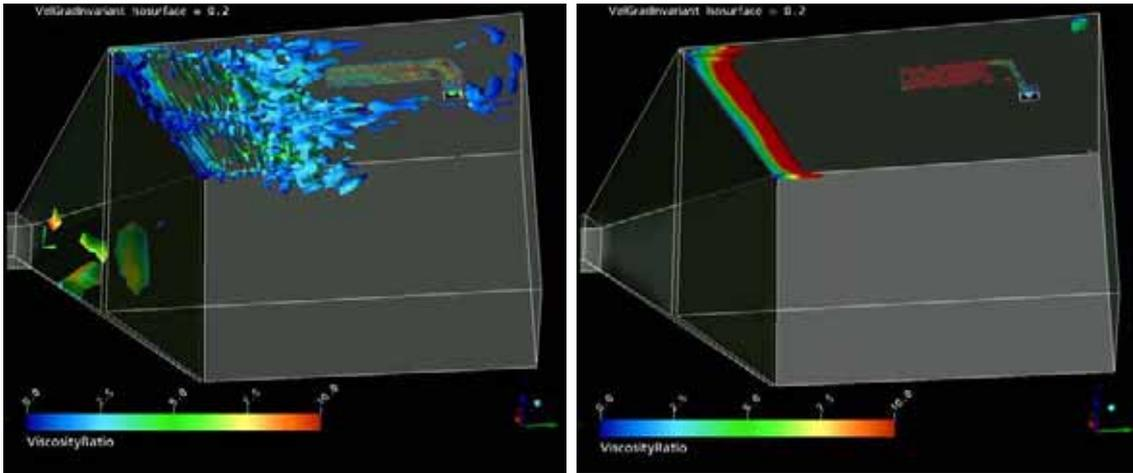
**Figure 6** Iso-contours of the velocity gradient invariant,  $I = 0.2$ , for the LES (left) and RANS model (right). Contours are coloured with the ratio of turbulent to laminar viscosity.
