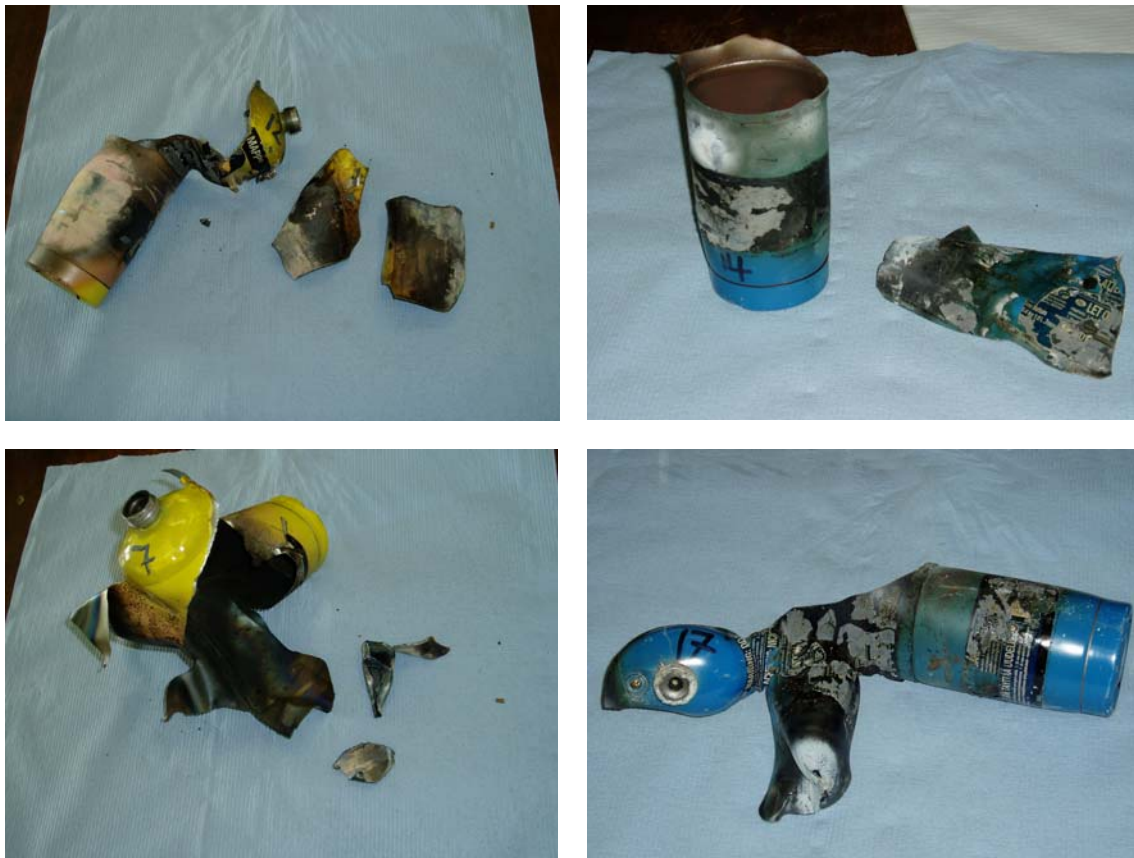
Figure 9: Photographs of failed cartridges from Test Series D.
