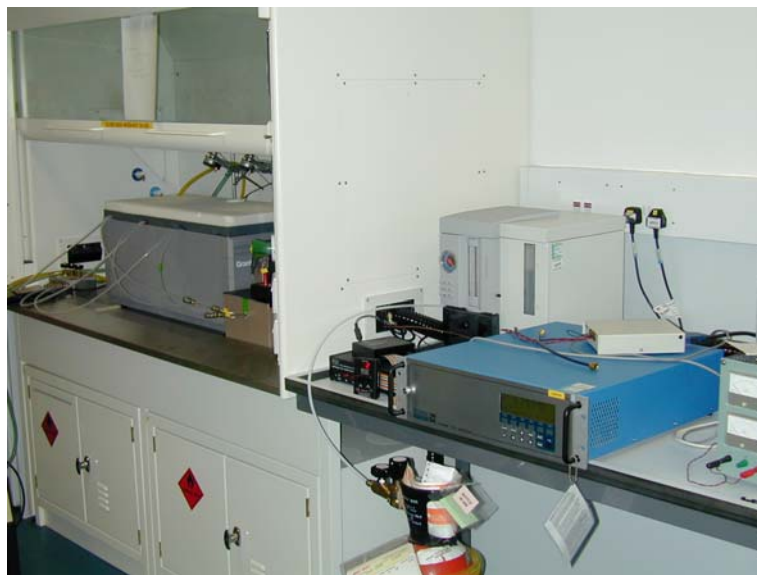
Figure 5.3. Glove testing rig, showing FID to the right.
