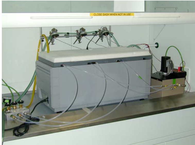
Figure 5.2. Glove testing rig, showing modified water bath and valve.
