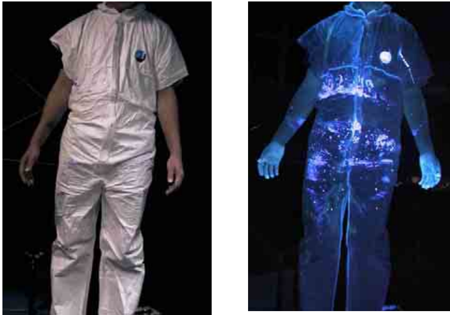
Fig 5. Oversuit under normal and UVA light showing heaviest spread of solvent and also the presence of flock on the hands
