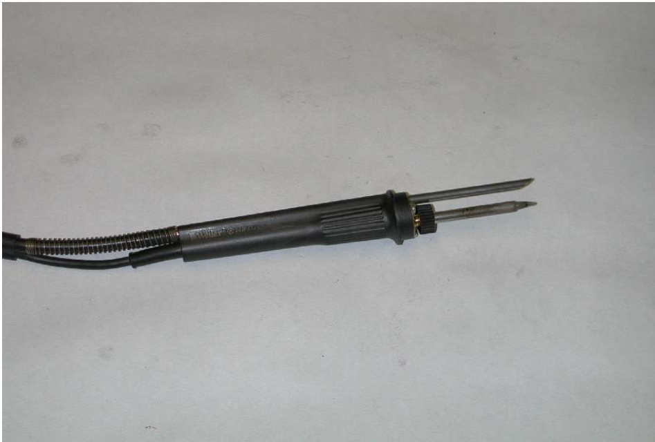
Figure 1.1: Soldering Iron with Tip Extraction Pipe as Supplied by Weller
