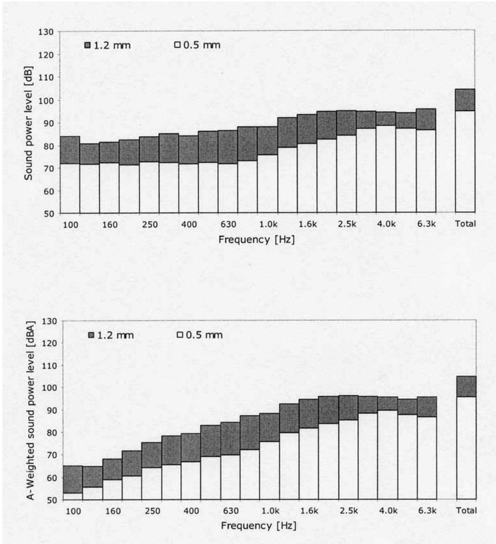
**Figure 16** Linear and A-weighted sound power one-third octave band levels
