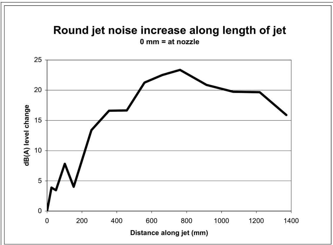
**Figure 6** Graphical display of A-weighted level change (Table 5 results)
