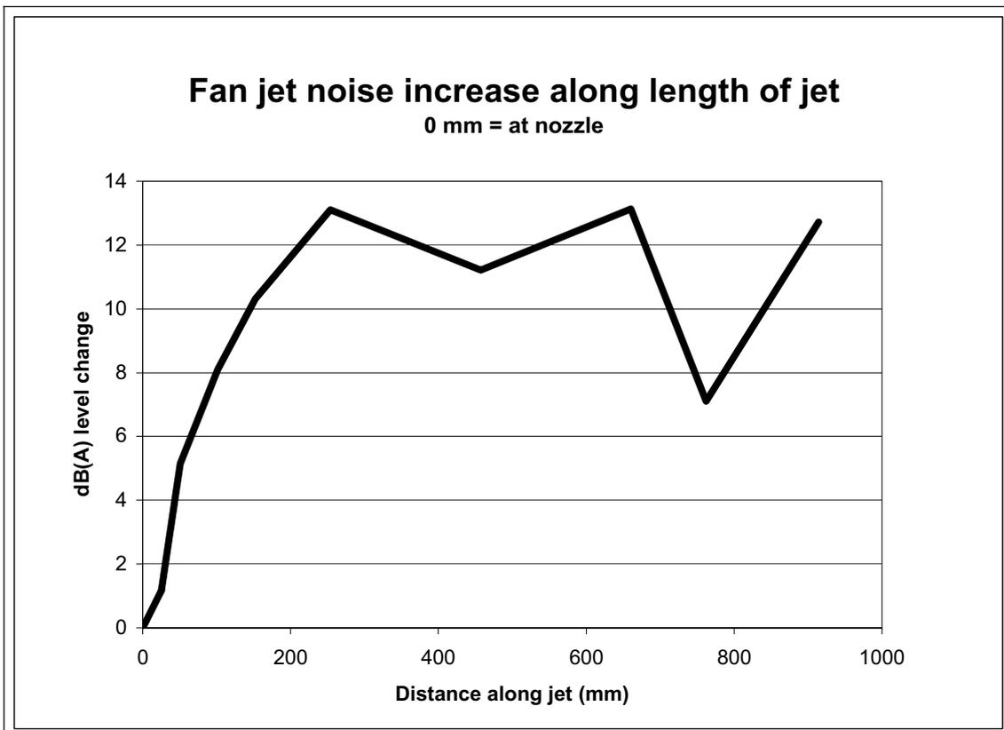
**Figure 7** Graphical display of A-weighted level change (Table 6 results)
