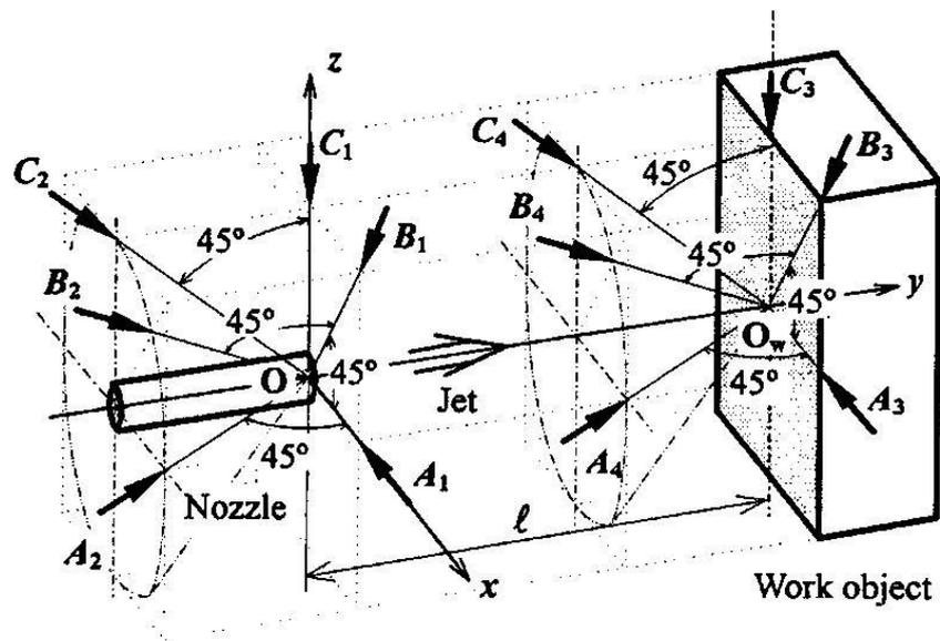
**Figure 18** Noise measurement microphone positions
