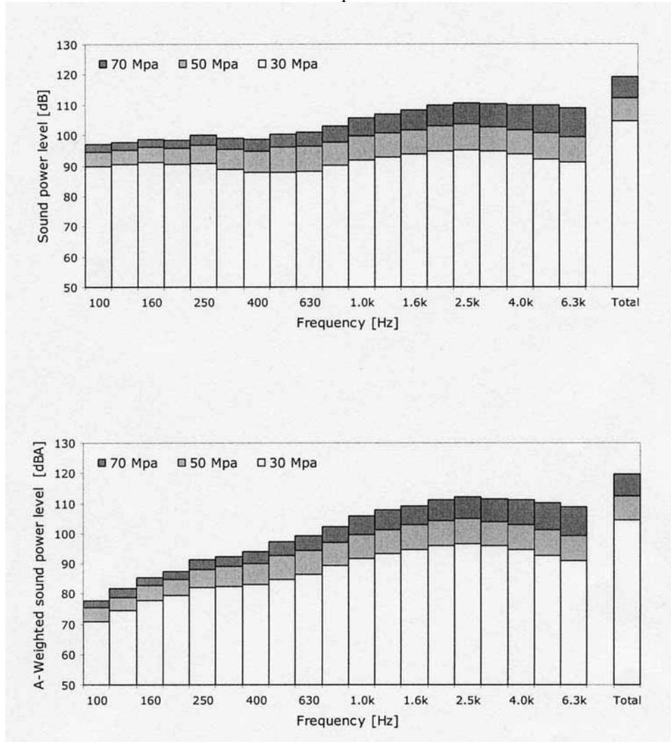
**Figure 14** Linear and A-weighted sound power levels
