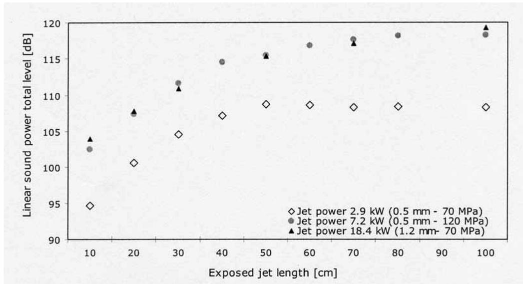
**Figure 17** Overall linear sound power levels vs exposed jet length
