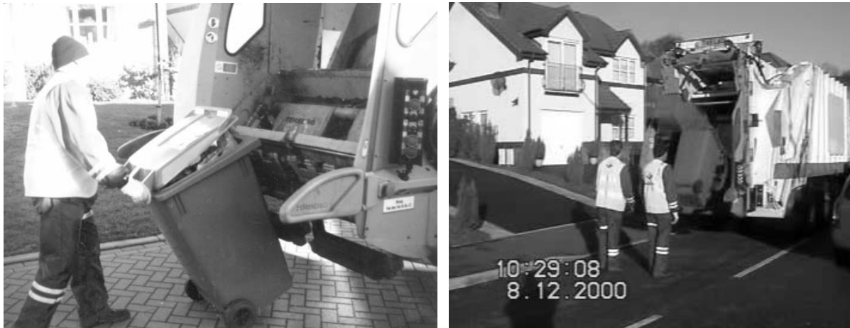
Figure 40. 240 litre green bin being pushed onto bin lift
