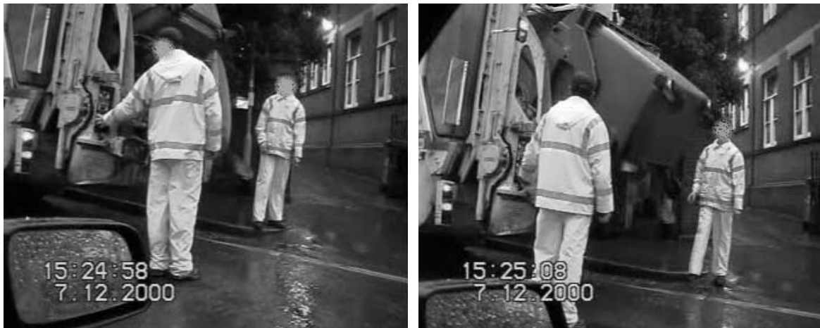
Figure 50. Shaking and lowering of 1100 litre bin
