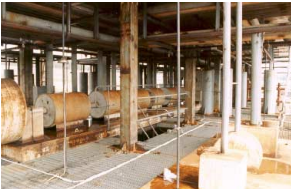
Figure 17: Internal view of full-scale rig used for Joint Industry Project on offshore gas build-up
