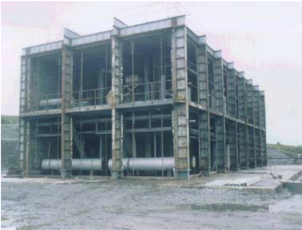
Figure 16: External view of full-scale rig used for Joint Industry Project on offshore gas build-up
