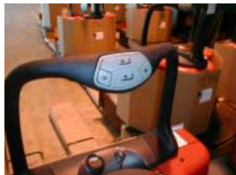
Figure 5: Showing grab rail and rabbit speed selector buttons on pedestrian/stand-on trucks
