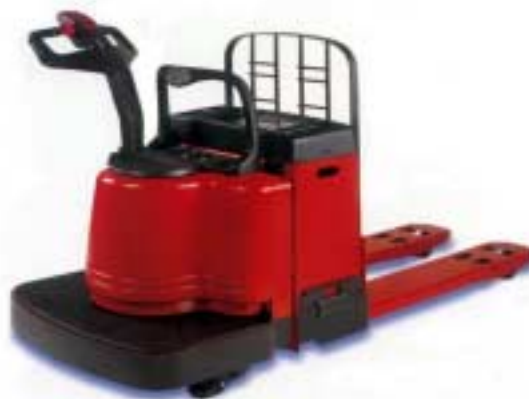
Figure 3: Pedestrian/stand-on pallet transporter (USA Style – fixed end platform)
