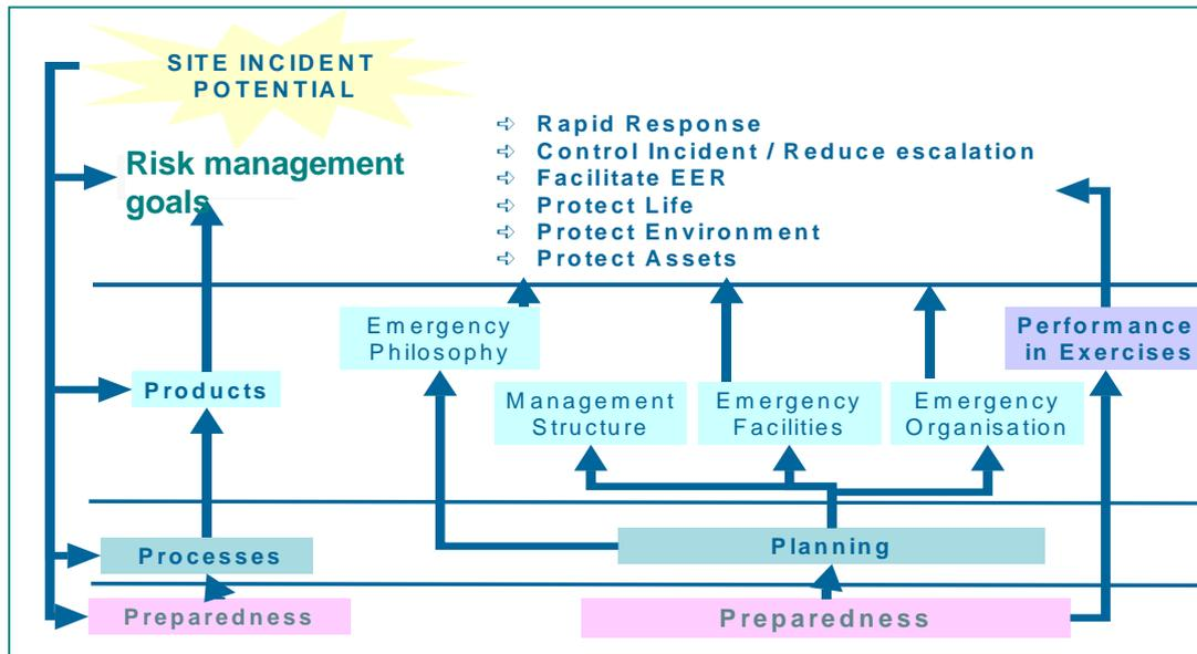
Figure 1 shows the structure of the EMPIRE system, and how the effectiveness of emergency management can be measured by examining the Risk Management Goals. These goals address the site hazards and the potential for major accidents at an installation and the company’s strategy for dealing with emergencies arising from such events.
