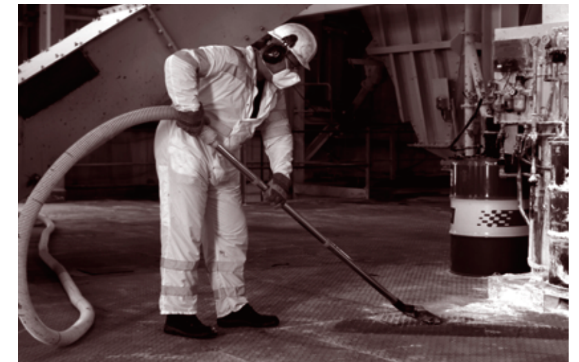
Dust spillage should be contained and vacuumed, not swept with a broom
