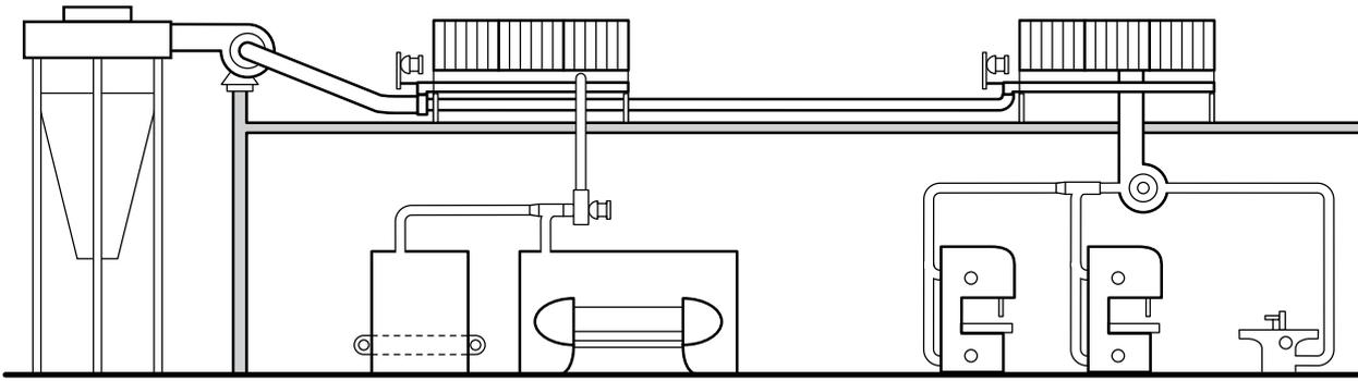
**Figure 2** Typical dust extraction system
