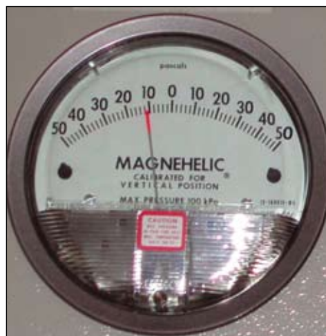
Figure 14 Example of a manometer fitted to a spray booth
