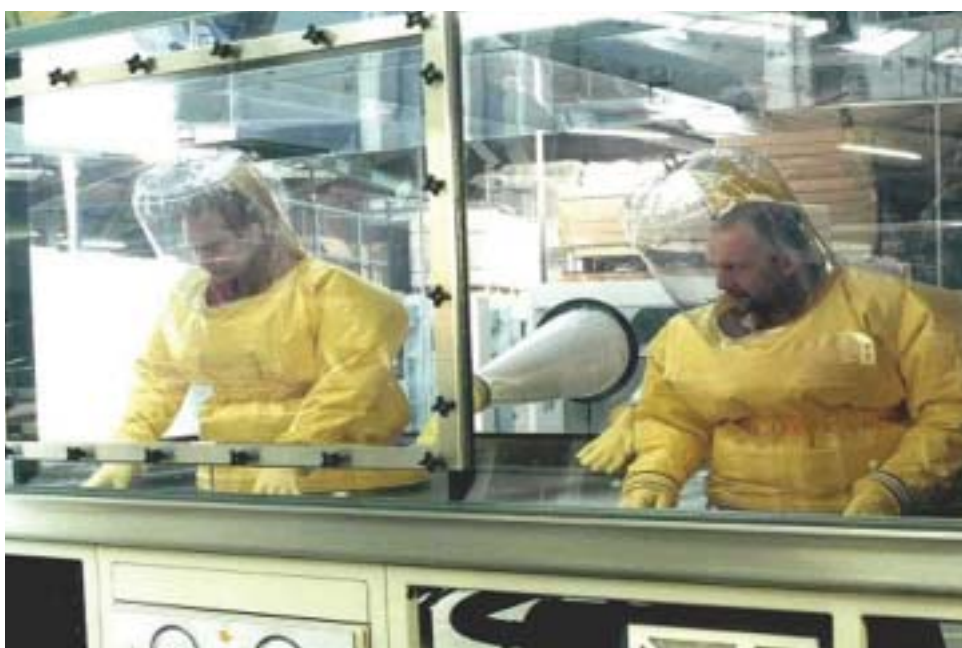
Figure 6: An example of a half-suit animal isolator
