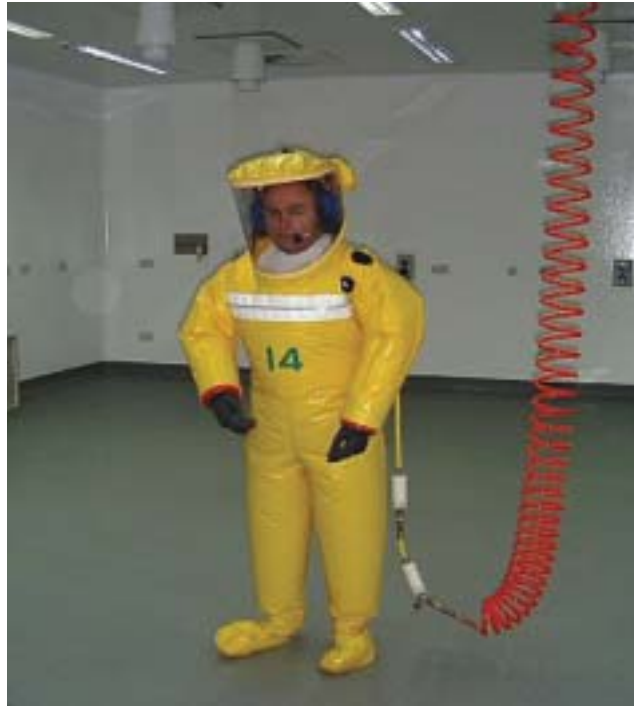
Figure 5: An example of a positive-pressure air-fed suit
