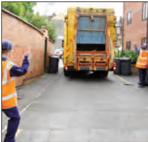
When aiding the driver reverse in a straight line, the reversing assistants should be positioned in a staggered pattern.
