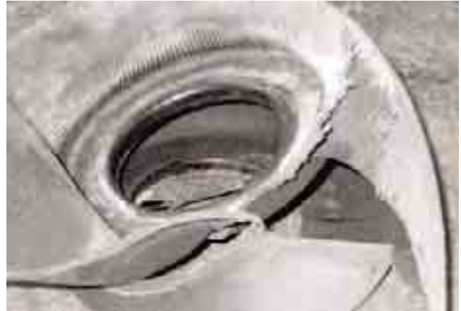
Figure 7 Typical bellows that has been over inflated
