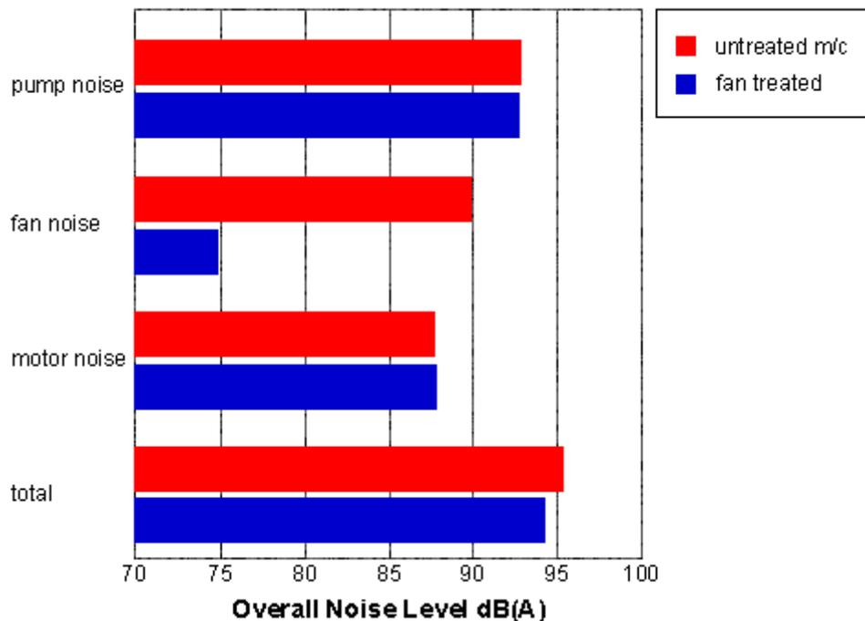
If it is assumed that the fan is the noisiest source (due to the subjective impression caused by tonal content) without carrying out the ranking process, and a silencer is fitted, then the result is as shown above. A 15 dB reduction in the fan component only produces a 1 dB overall noise reduction as it is not the dominant source. Used properly, the ranking process allows the overall noise reduction to be estimated in advance before spending money on modifications.
