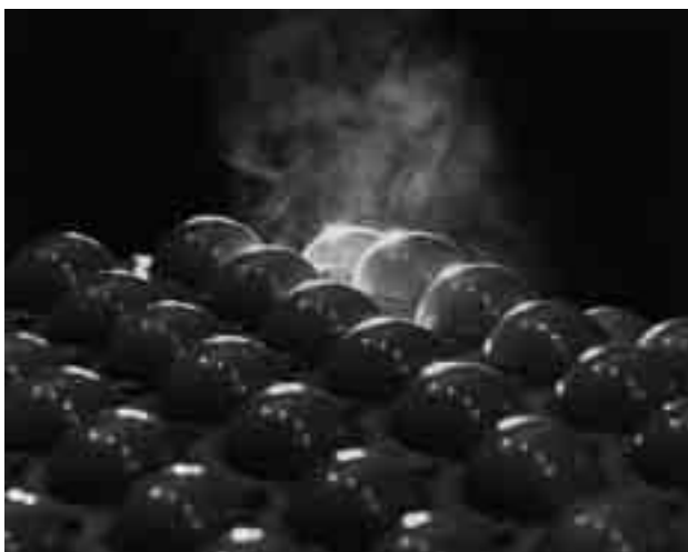
Plate 3 Rubber fume is revealed using the dust lamp
