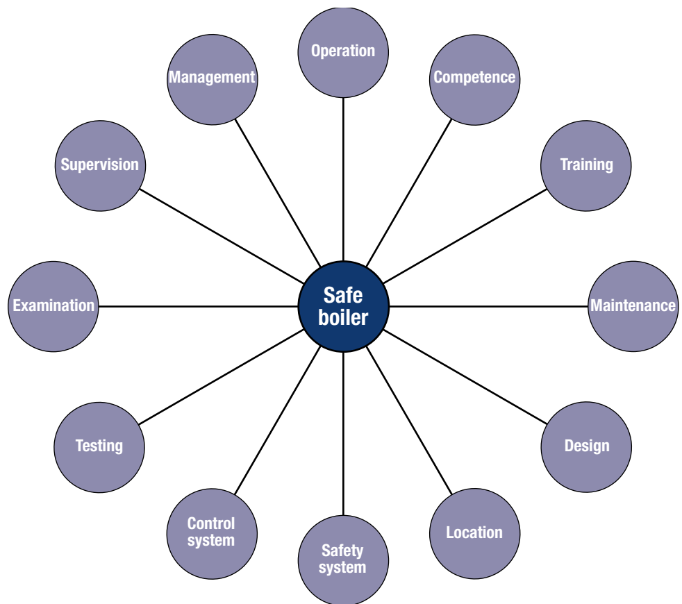
Figure 3 What can affect safe boiler operation?
