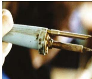
**Figure 2** On-tool extraction – soldering iron
