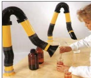
**Figure 5** Moveable capturing hood
