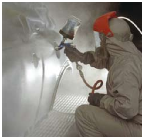
'Now you see it...' Special lighting and black background show paint mist enveloping sprayer
