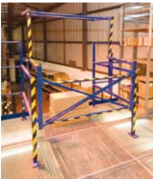
A pivoting safety barrier ensures the fence opening is guarded at all times
