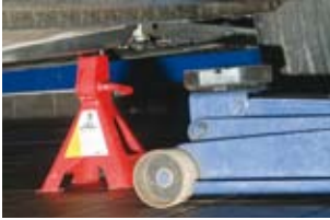
Always use axle stands if working beneath a vehicle raised on a jack
