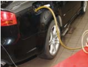
A fuel retriever showing mechanical pump and earthing cables
