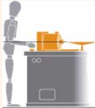
Figure 3 Checking lathe for correct working height
