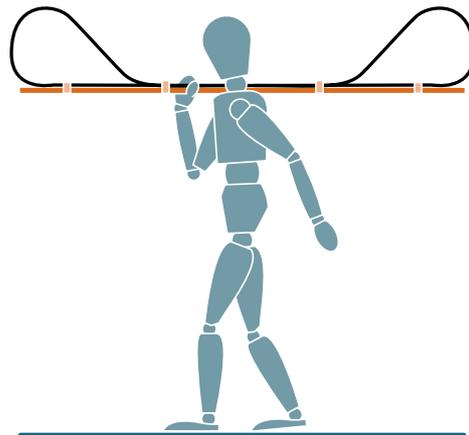
**Figure 3** Band saw blade transit board
