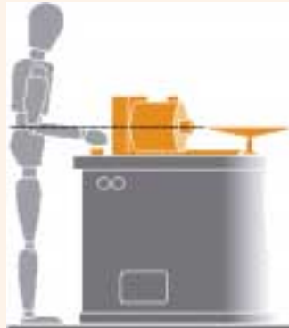
Figure 3 Checking lathe for correct working height
