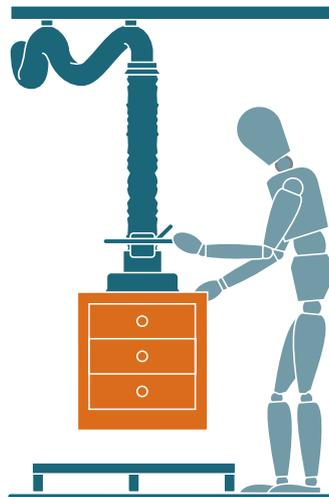
**Figure 7** Vacuum-handling device
