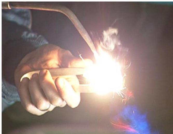
**Figure 3 Spark ignitor**
