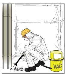
It is important to note that generated dusts may also contain specific airborne contaminants from the existing paint (eg lead, chromium etc) and exposure should be controlled within the exposure limit for each contaminant. Specialist advice should be sought for these situations.
