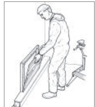
Use non-asbestos boarding to protect asbestos
