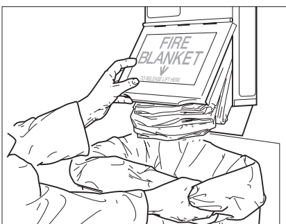
Open the front, dampen, and slide the blanket into the waste container
