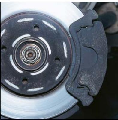
Disc brake on a vehicle
