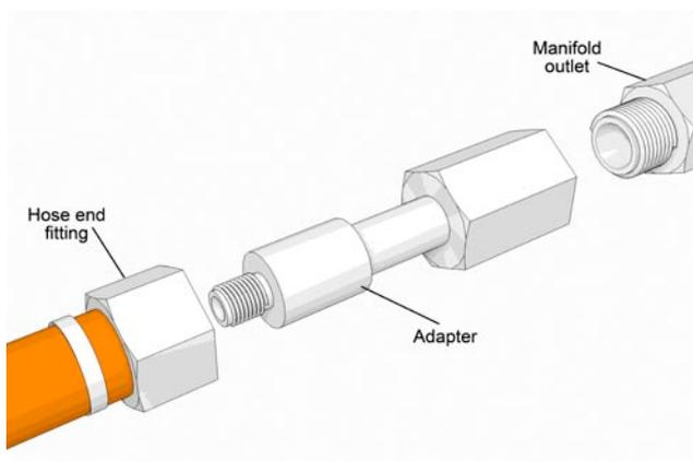
**Figure 2** Suitable arrangement for use of an adaptor
