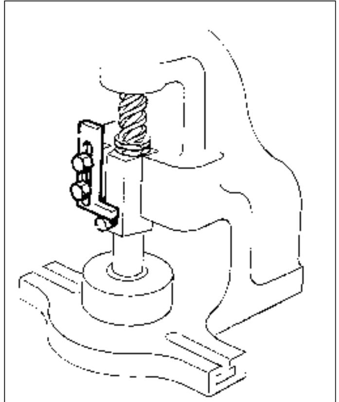
**Figure 3** Restricted stroke device
