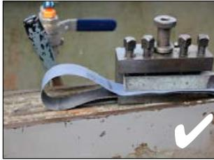
The tool post is used to clamp and hold a looped strip of emery cloth in place during application (see video demonstration at [www.hse.gov.uk/engineering/lathes.htm](http://www.hse.gov.uk/engineering/lathes.htm)). This method is for external deburring work only. It almost entirely eliminates the risk of injury.
