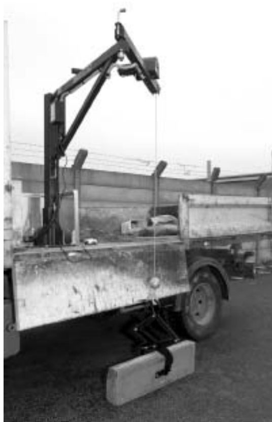
Figure 2 Vehicle-mounted crane and mechanical grab
