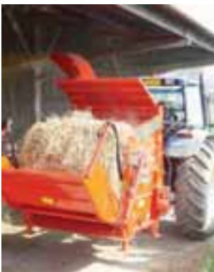
Figure 7 Tractor-mounted straw chopper for spreading fresh bedding
