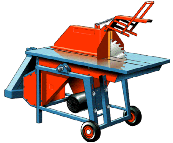
Figure 1 Cross-cut saw with log gripper
