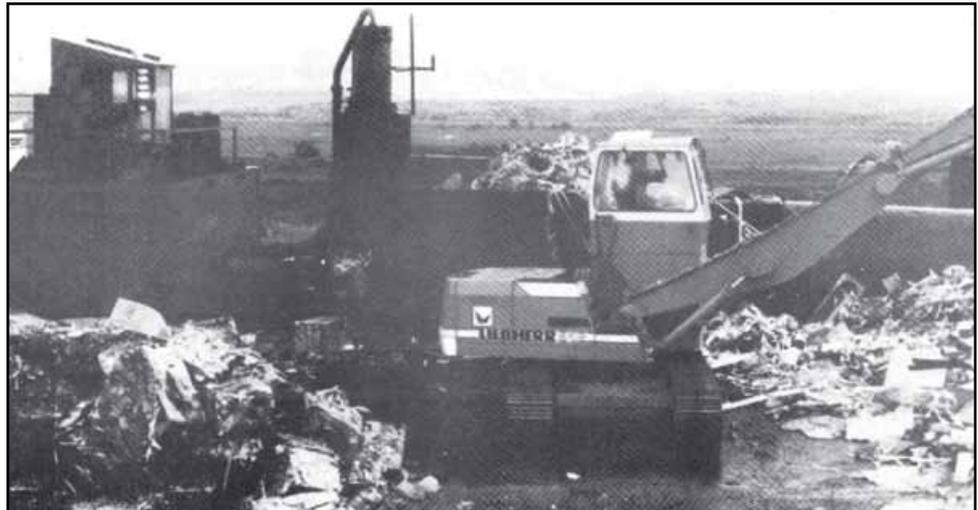
**Figure 3** Large baling machine - radio controlled. Note lights at side of original control cabin indicating state of baler. Complete operation controlled by crane driver.
