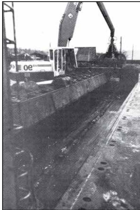
**Figure 1** Large baling machine showing rail protection at edge of platform near control cabin
