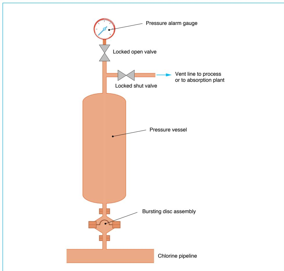
54 New steel pipework should be pressure tested to at least 12 bar gauge using dry (dew point less than -40°C) air, nitrogen or any other suitable gas. Any
