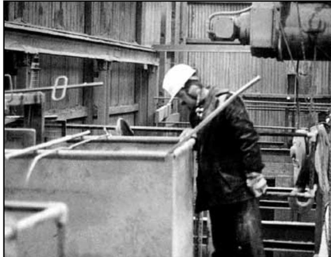
**Figure 5** Secondary crusher before modification (107 dB(A))
