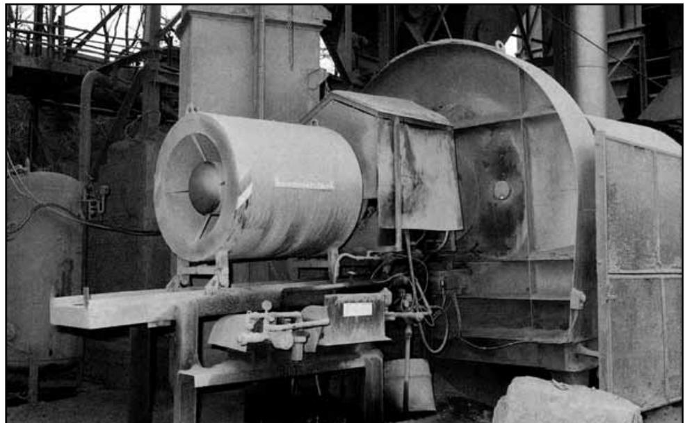
**Figure 8** Use of silencer on burner
