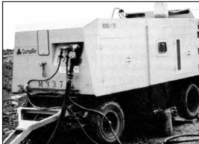
**Figure 3** New 'silenced' compressor
