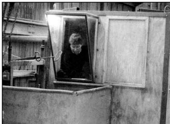
**Figure 6** Secondary crusher after modification (81 dB(A))
