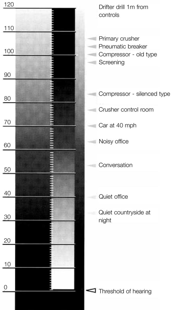
**Figure 1** Some typical dB(A) noise levels
