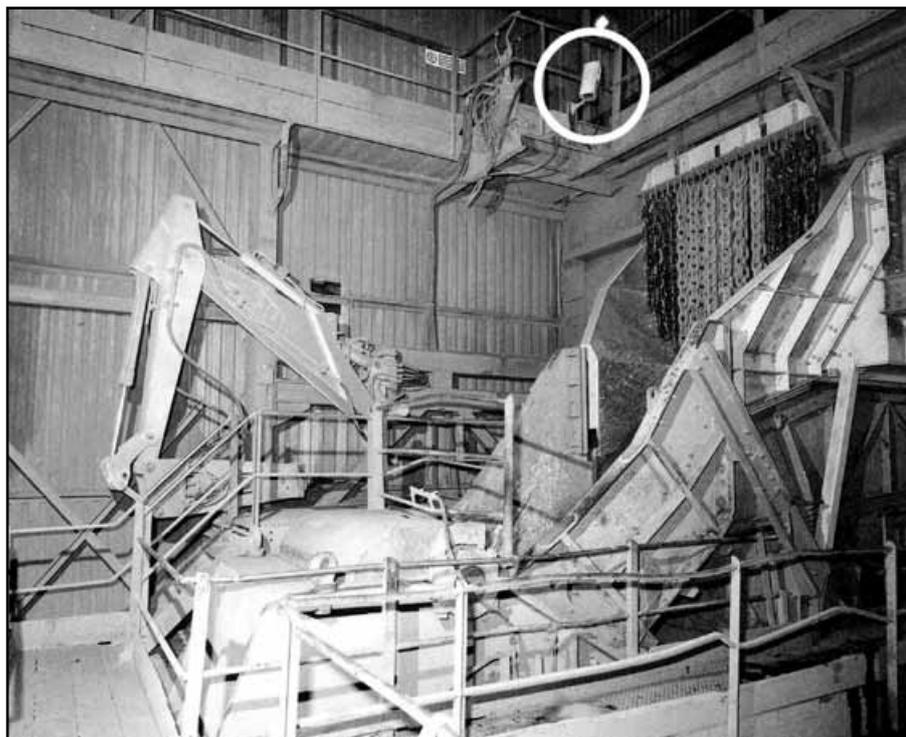
**Figure 4** CCTV camera in use at a primary crusher (ringed)
