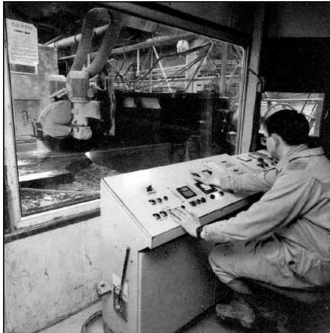
**Figure 9** Remote/automatic control of saws
