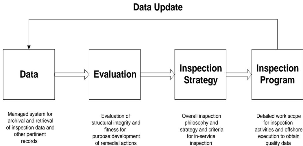
Figure 3: Structural management cycle from ISO 19902 [5]
