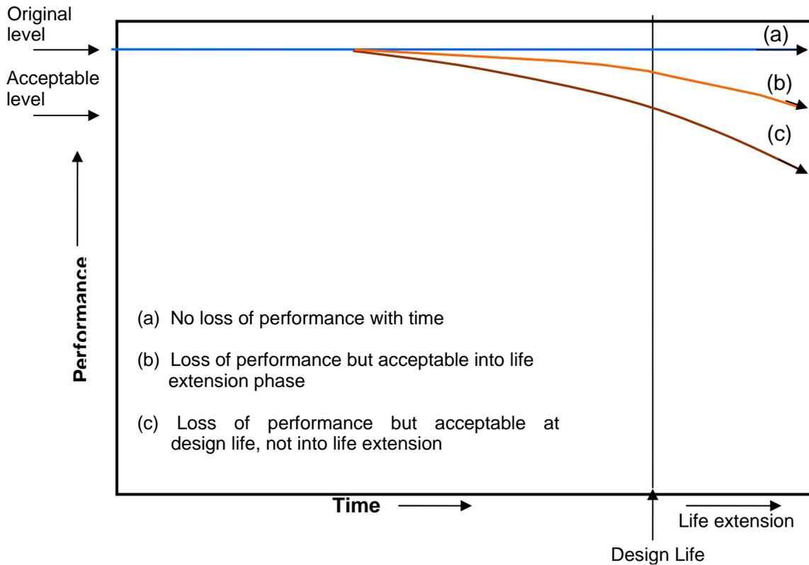
Figure 2: Structural performance during life extension phase
