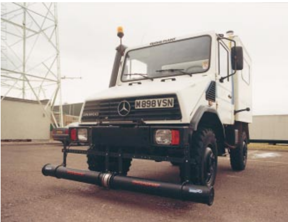
New 'Groundhog' beach monitoring vehicle
