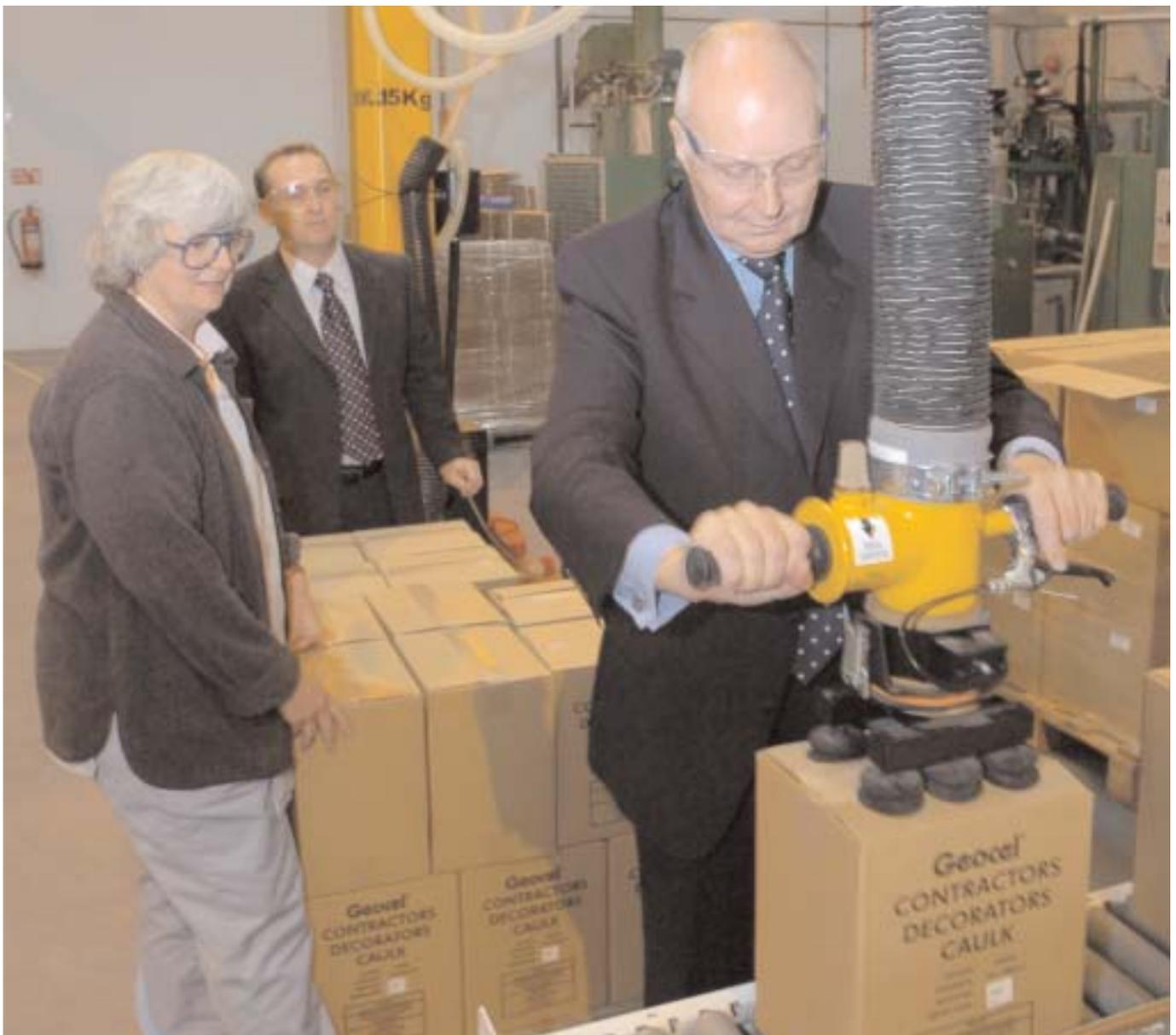
*Will Barclay, Managing Director, operating the box vacuum lifter, a device used to reduce manual handling of heavy boxes*
