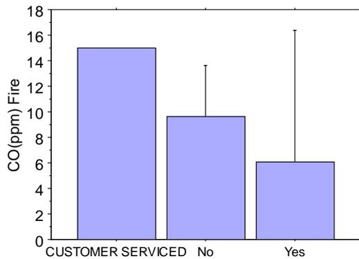
**Figure 11 : Mean carbon monoxide concentrations measured from Gas Fires (main room) split by maintenance in the last year or not.**
