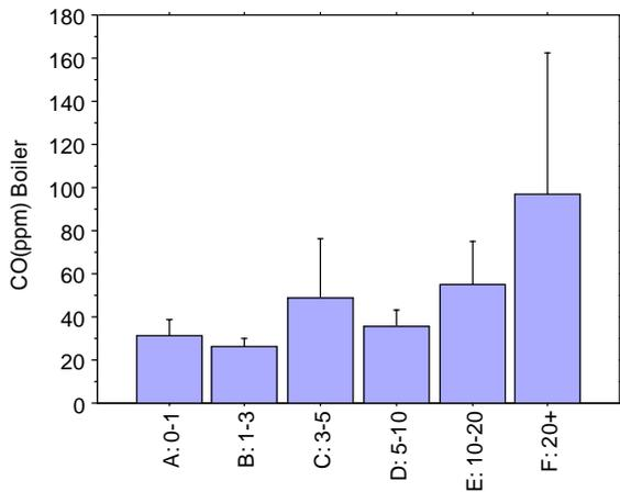
**Figure 6 : Mean carbon monoxide concentration measured from boilers split by their age range.**
