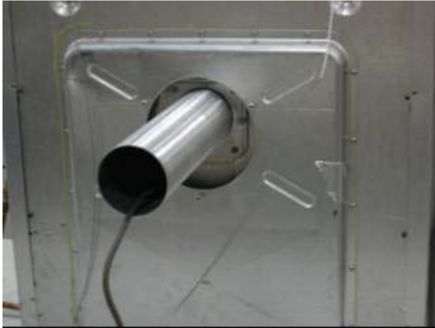
Figure 11: Location of the sampling probe in balanced flue fire
