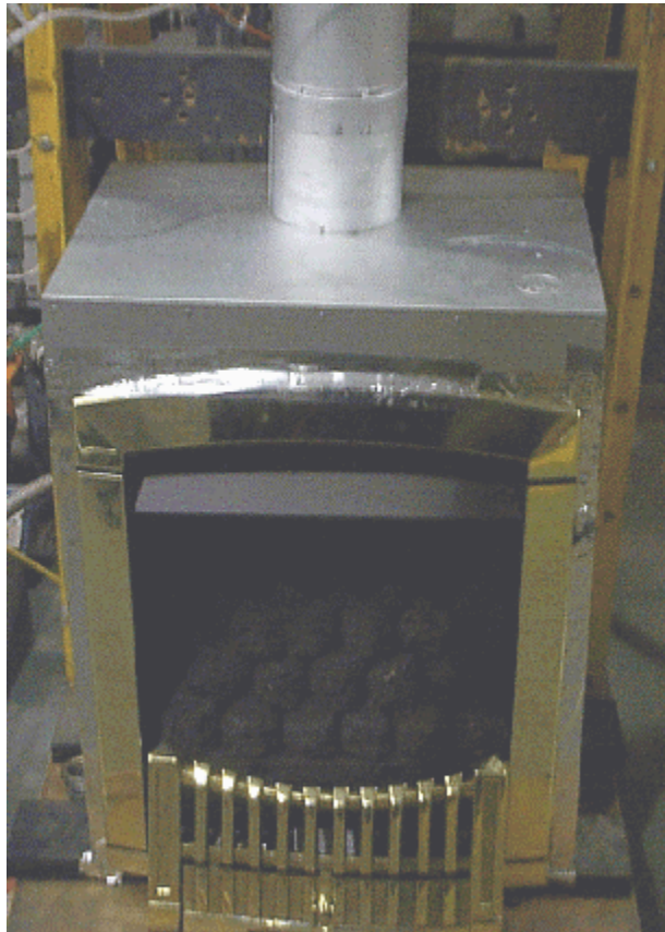
Figure 19: Open flue coal-effect inset gas fire
