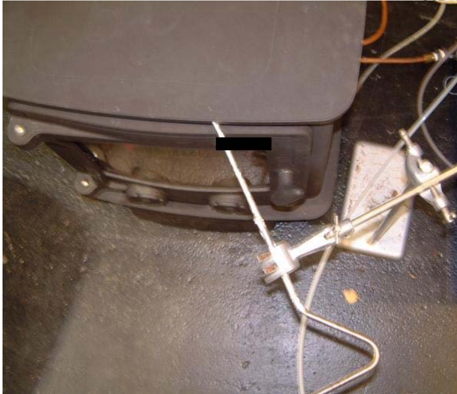
Figure 4: Position of external sample probe from above
