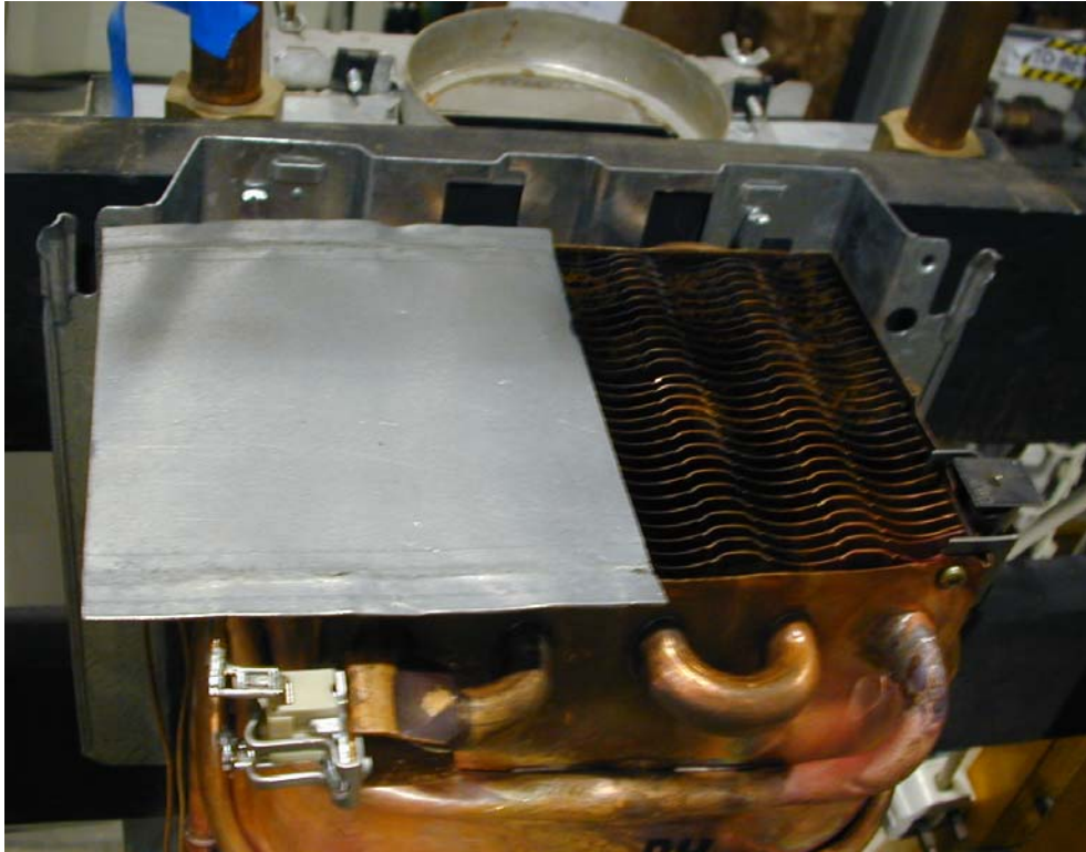
Figure 17: Blockage of water heater heat exchanger
