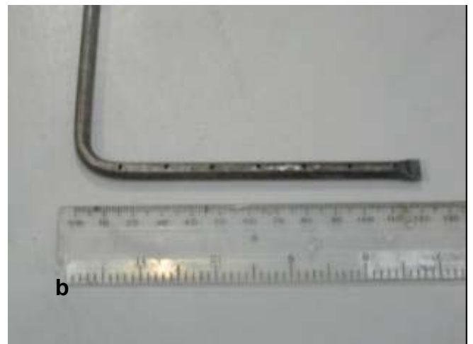
Figure 3: Detail of two multi-point sample probes
