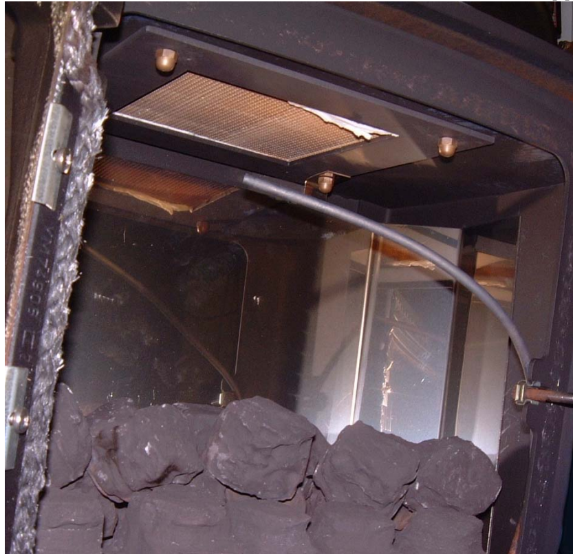
Figure 6: Position of internal sample probe (1)
