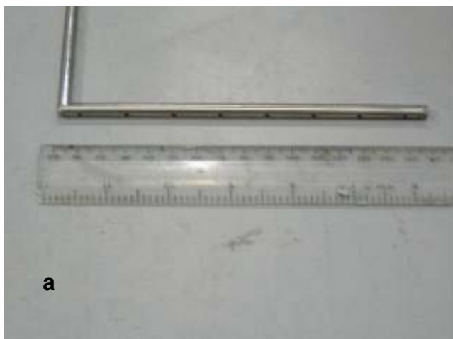
Figure 3: Detail of two multi-point sample probes
