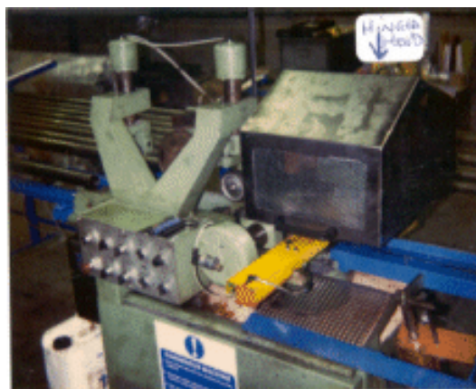
Photograph 3: Automatically fed Type A machine showing fitted additional hinged, interlocked hood guard to prevent inadvertent access to saw blade.
