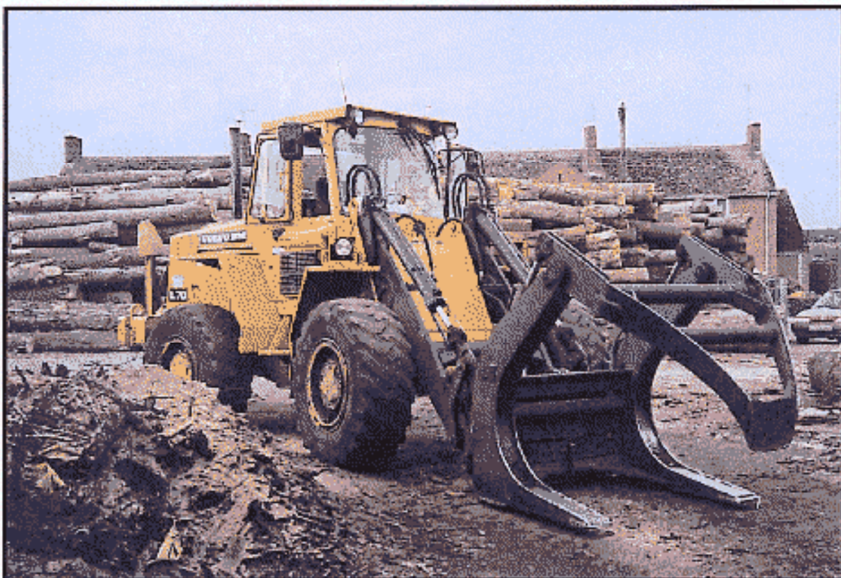
Figure 6 - A wheel loader with grabber attachment.
