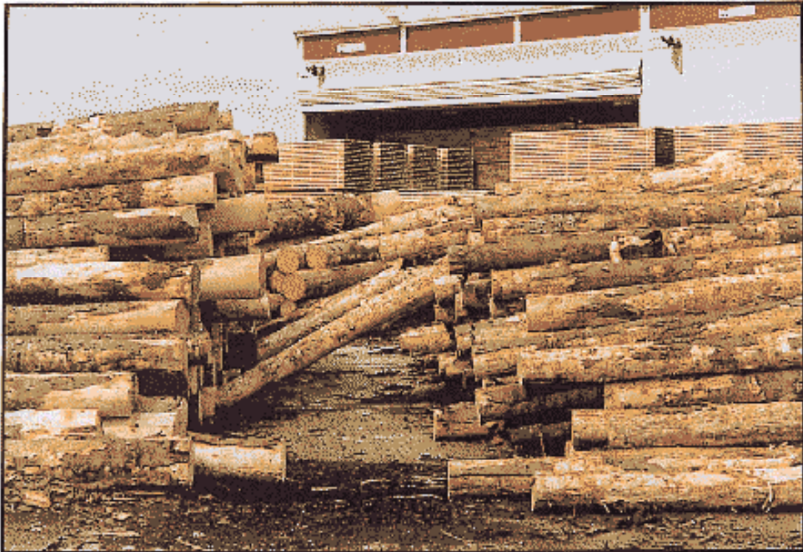
Figure 12 - Slippery logs which have slipped off the stack.
