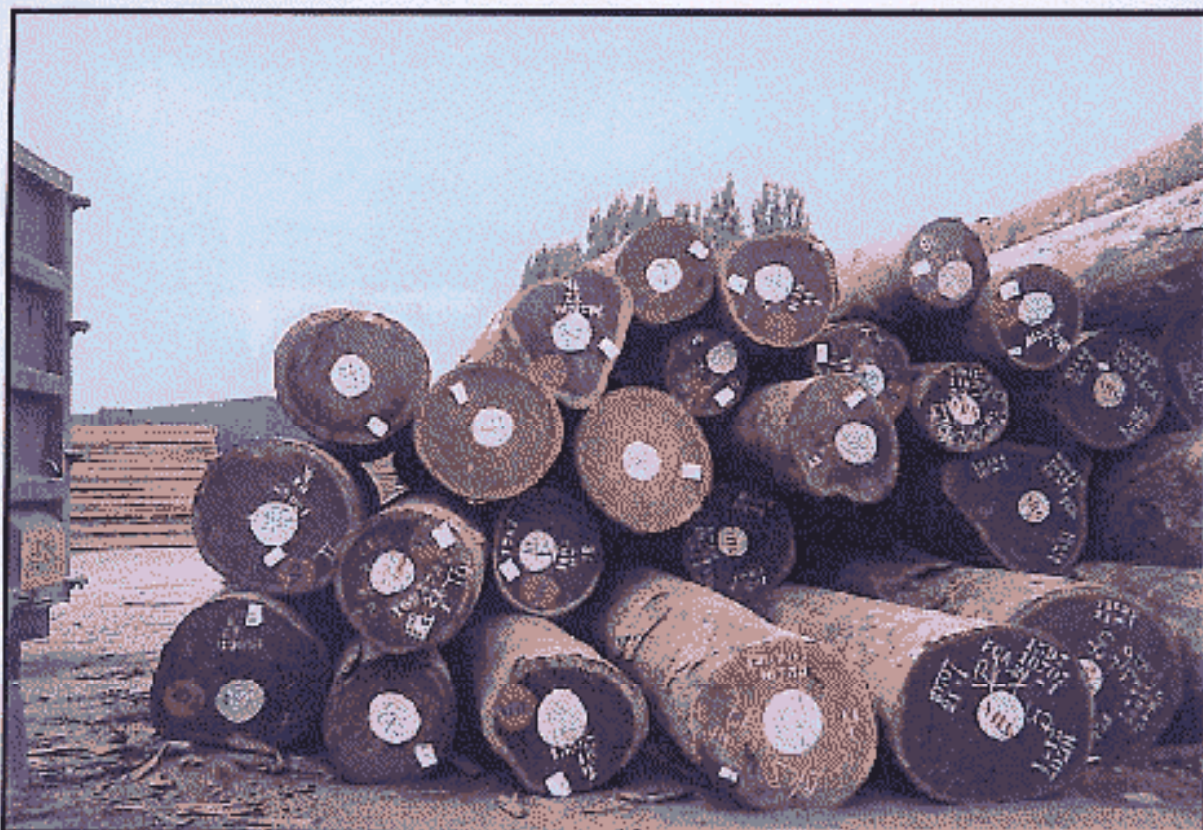
Figure 16 - Hardwood logs stacked with a steep end angle.
