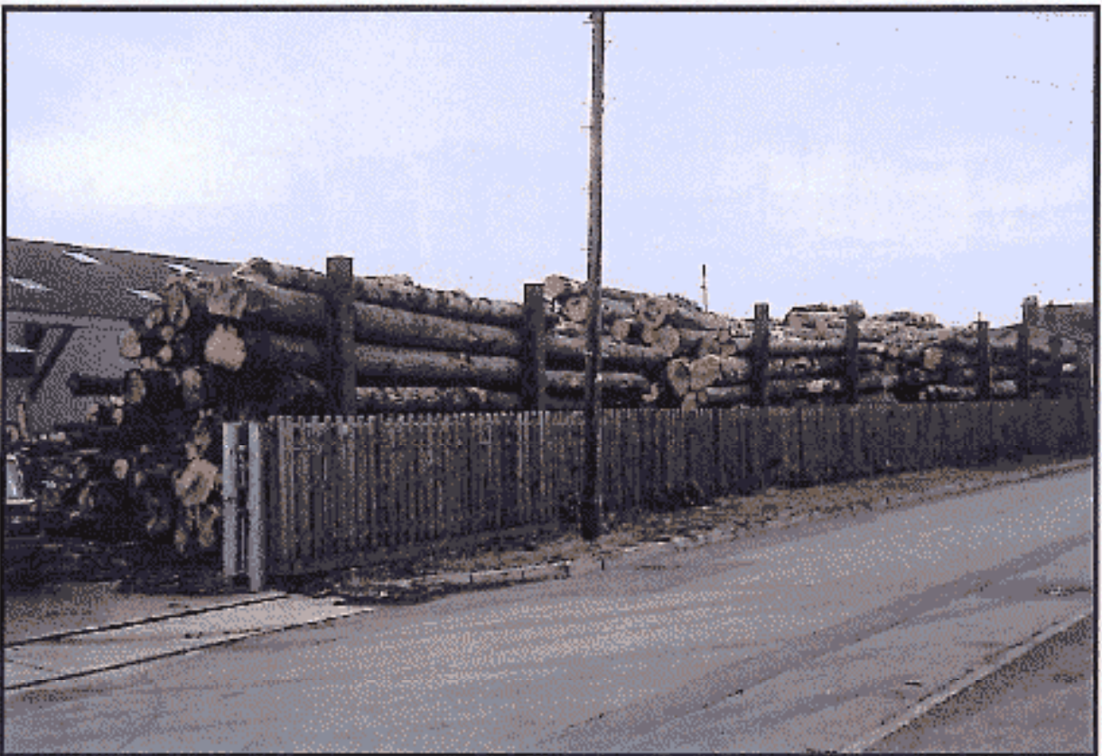
Figure 4 - Supports for one end of log stacks - the boundary next to a public road.
