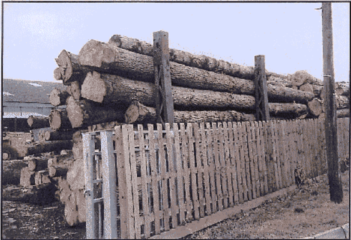
Figure 3 - Supports for one end of log stacks.
