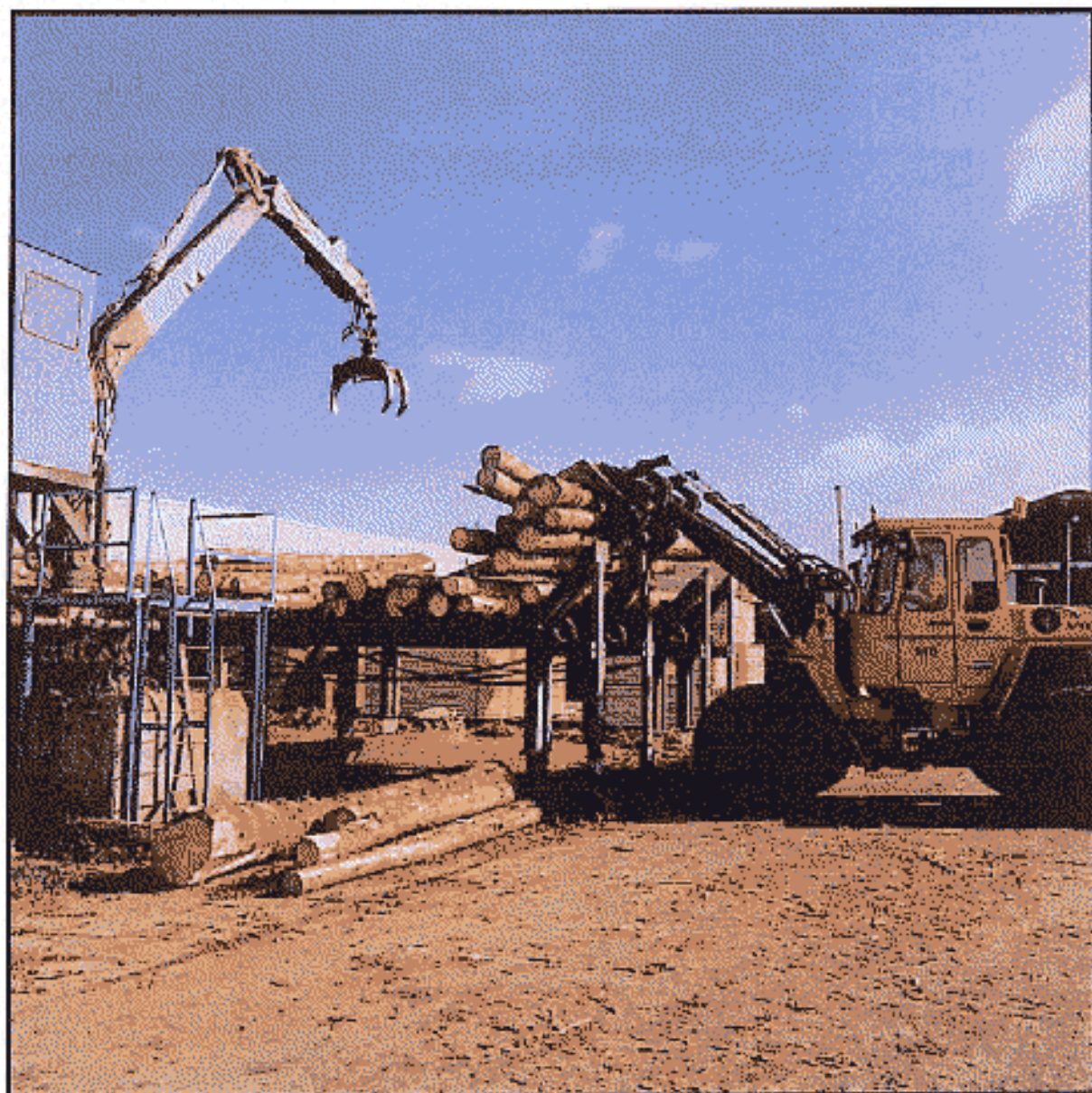
Figure 20 - Feeding a mill with a wheel loader.
