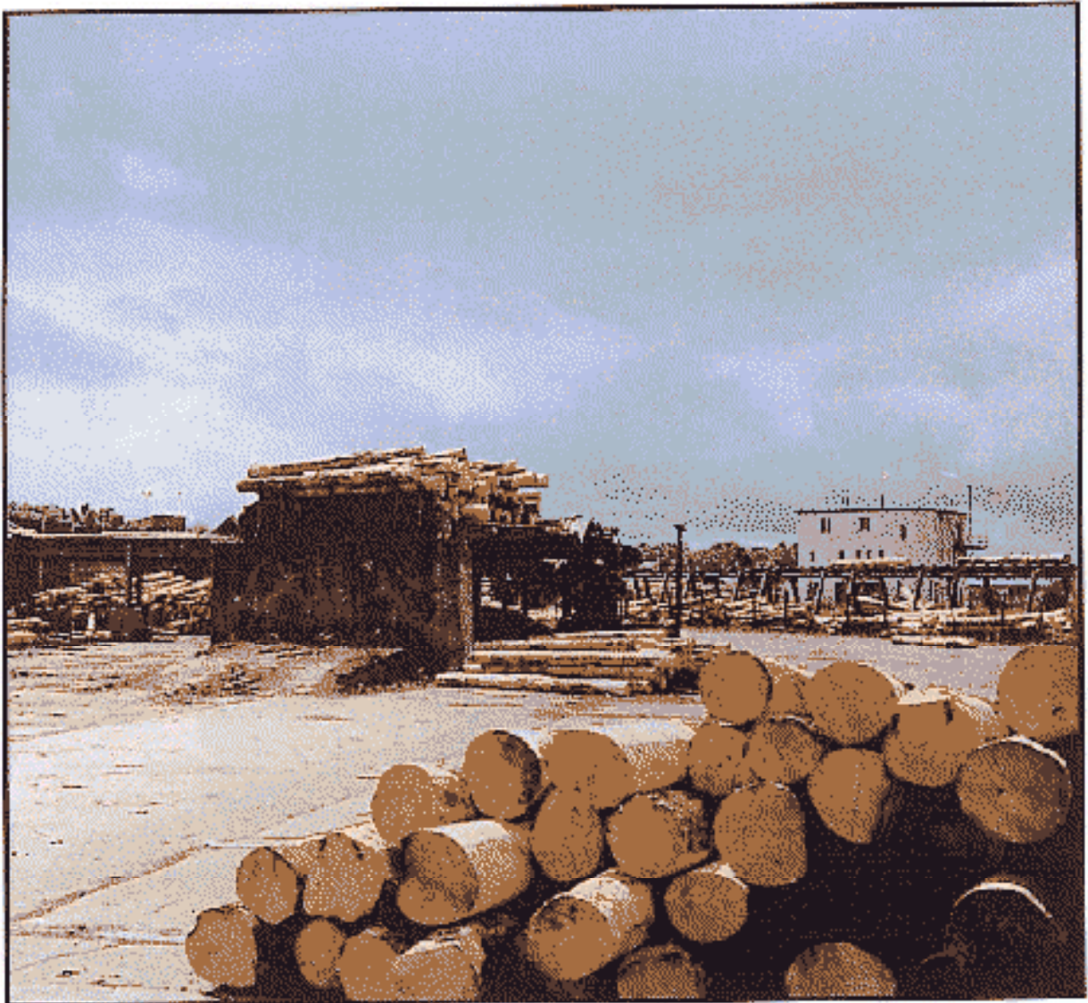
Figure 21 - The loading deck for a mill which is too high for a shovel loader.
