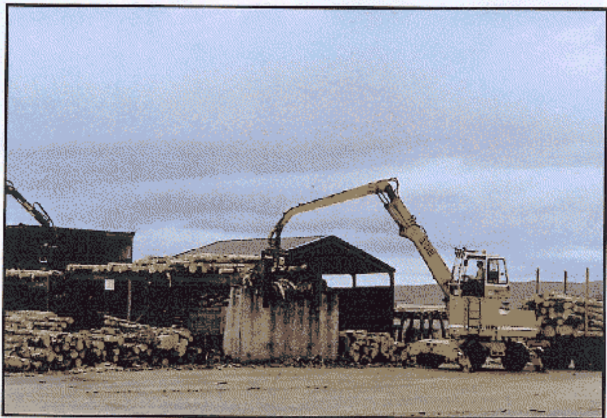
Figure 19 - Logs being fed into the mill using a mobile grabber with rotary jaws.
