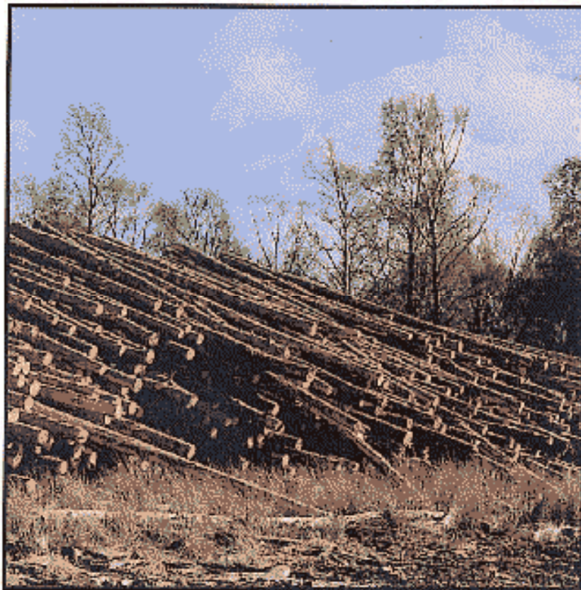
Figure 14 - Long logs with butt ends to one side of the stack.
